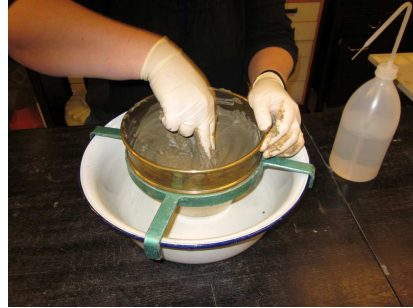
Figure 5.2 Grating the clay to maximise the surface. Figure 5.3 Pugging the clay through a 0.42 sieve.
