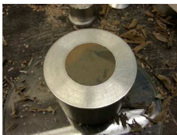
Figure 6.6 A levelled sample, the variation in colour is evident.
