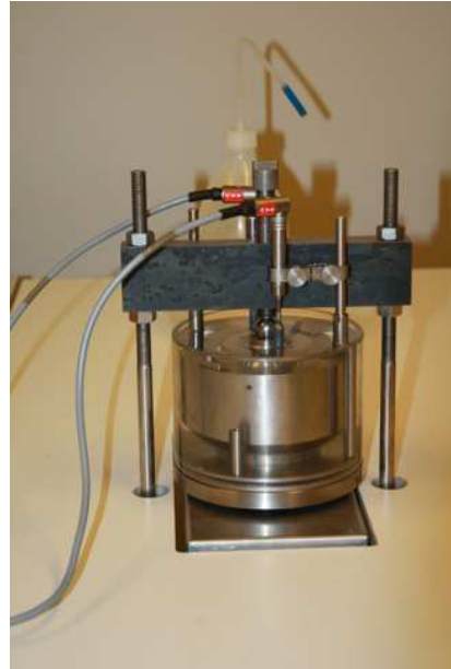
Figure 6.3 Danish incremental loading oedometer apparatus.
