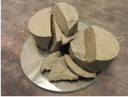
Figure 1: Fissured structure of a Søvind Marl sample. Sample diameter is 72 mm.
