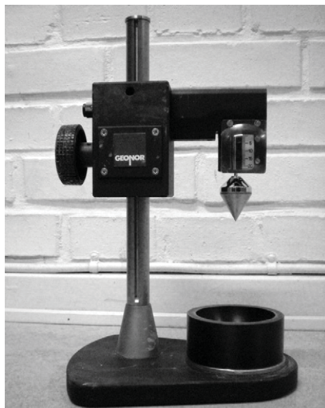
Figure 3. The Fall Cone Apparatus used for the tests.
