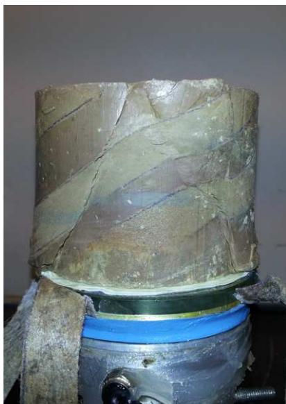
Figure 7.8 Test 6 after shearing.
