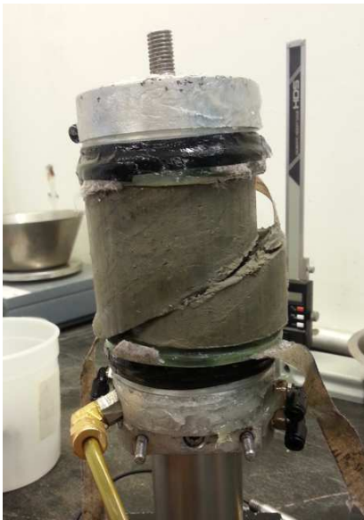
Figure 7.6 Test 4 after shearing.
