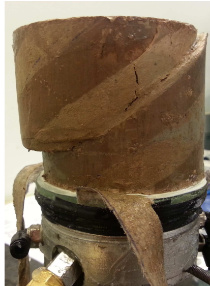
Figure 7.5 Test 3 after shearing.
