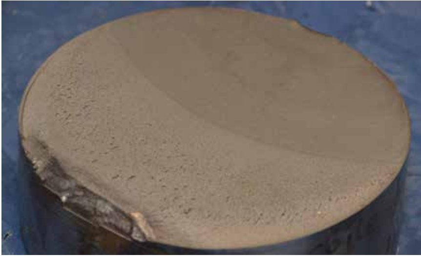
Fig. 4.1: Fatigue failure of a steel shaft which has been exposed to a bending moment and rotation, similar to loading of train shafts.
