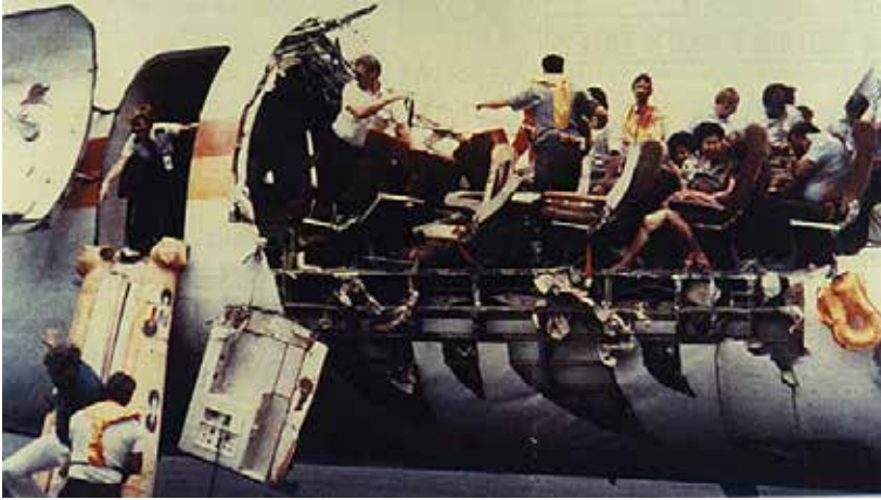
Fig. 1.3: Fatigue failure in a Boeing 737-200 from Aloha Airlines Flight 243 which operated near Hawaii. "Winnipeg Free Press, Saturday, May 21, 1988".
