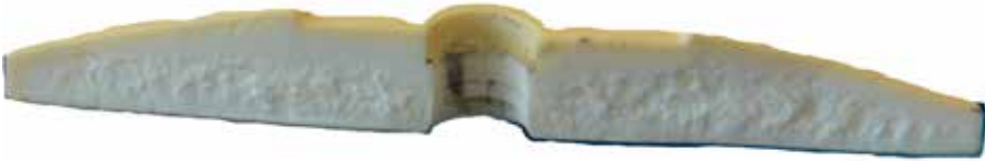
Fig. 4.11: Polymer application with failure caused by stress oscillation.
