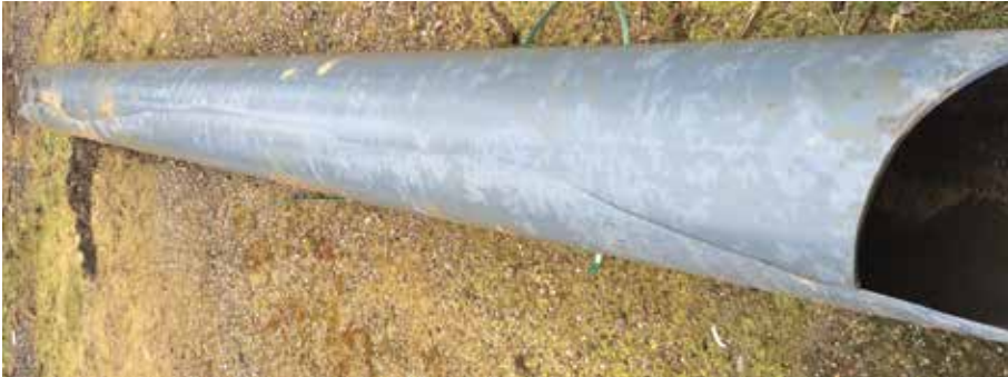
Fig. 4.15: Failure of a \varnothing 400 mm PVC pipe in a water distribution system under long-terms loading by water pressure.
