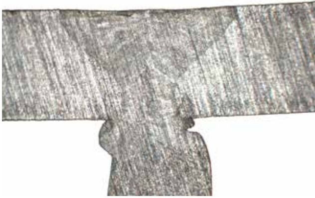
Fig. 5.6: Laser welding of AISI 304 in a T-joint configuration.
