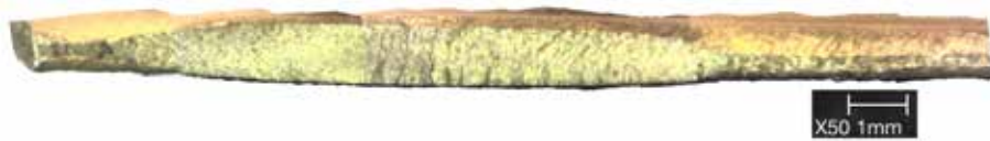
Fig. 3.14: Fracture surface of a specimen of AISI 304 laser welded T-joint.
