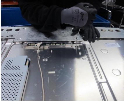
Picture 11-4: Disassembly of the television; the printed circuit board is sealed off by several metal plates held together by screws and it is therefore both time consuming and difficult to remove them manually
