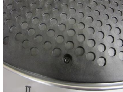
Picture 11-18: Screw submerged in plastic.
