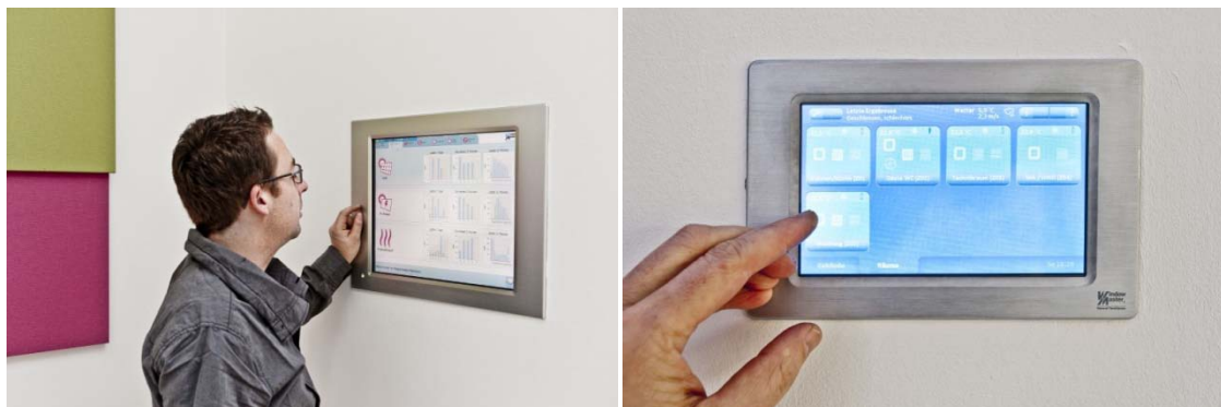
Figure 3. MWa Touch screen. The main monitor screen in the house where data can be assessed and occupants can acquire feedback and change settings.
