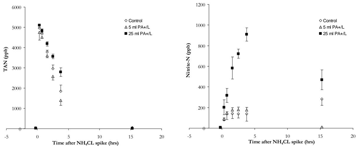
**Fig. 7.4. Evaluation of biofilter performance after exposure to Peraqua Plus (PA+).** PA+ (containing 12.5 % PAA and 34 % HP) were added to individual bioblok units (cylinder tube) in individual reactors (N=9) and after complete disinfectant decay, reactors were spiked with NH<sub>4</sub>Cl and simultaneous TAN and nitrite concentrations were measured. Ammonium removal ranged from 0.18-0.27 g TAN·m<sup>-2</sup>·d<sup>-1</sup> (L-F Pedersen; *unpubl. data*).
