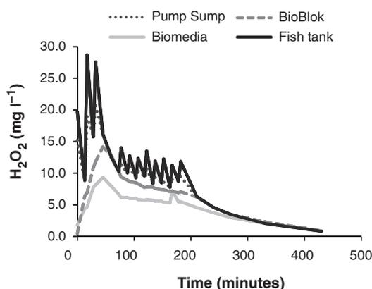
**Figure 11** Hydrogen peroxide (HP) application in recirculating aquaculture system-B. The pump sump represents the inlet to the two biofilters (submerged, fitted with BIO-BLOK<sup>®</sup>, and fluidized, Biomedica); HP measured at the outlets from the biofilters and in the rearing tank.
