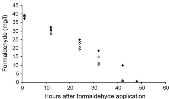
Fig. 3. Formaldehyde concentration in six closed pilot scale biofilters. Within 30 s ( $t_0$ ) 38.5 g formalin (37.5% (w/w) formaldehyde) was applied to each system, with an expected initial concentration ( $C_0$ ) of 40 mg formaldehyde/l. Solid symbols refer to experiment 7.1; open symbols to experiment 7.2–7.6 (cf. Table 2). Overall regression is described as  $y = 40.4 - 0.87x$  ( $R^2 = 0.95$ ).
