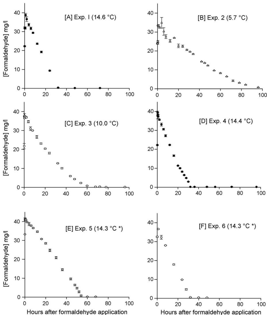
Fig. 2. Degradation of formaldehyde applied to a full scale biofilter at six different conditions. Temperature effects were investigated in experiments 1–4. (\*) In experiments 5 and 6, 40% of the total biofilter media was removed, and formaldehyde was applied immediately after removal (experiment 5) and reapplied after 2 weeks (experiment 6). A total of 906.7 g formalin (37.5% formaldehyde in 10% methanol stabilized solution) was applied to the system.
