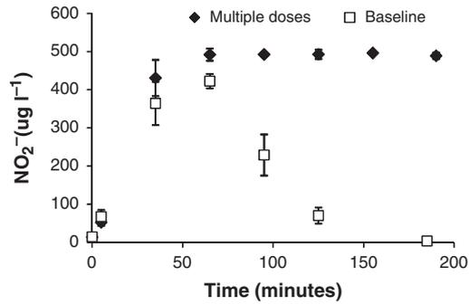
**Figure 6** Nitrite-N levels after multiple doses of hydrogen peroxide (HP) in recirculating aquaculture system (RAS)-A biofilter tubes. The 'baseline' shows the nitrite concentration in unexposed RAS-A biofilters and 'multiple H<sub>2</sub>O<sub>2</sub> doses' shows the nitrite concentration after multiple HP doses and complete HP removal. The data are the average from all six reactor tubes and the error bars represent the 95% confidence interval.
