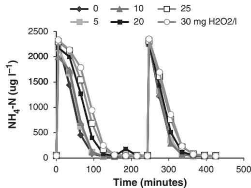
**Figure 9** Total ammonium nitrogen concentration in six biofilter tubes from recirculating aquaculture system-A after spiking with both NH<sub>4</sub>Cl and different initial hydrogen peroxide doses. NH<sub>4</sub>Cl was respiked at  $t = 240$  min.
