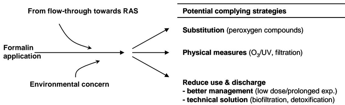
**Fig. 1.** A diagram illustrating the two main factors influencing formaldehyde application, and potential measures to comply with regulations. Biofilters are central treatment units in recirculating aquaculture systems (RAS), where water is recycled as opposed to traditional flow-through systems.
