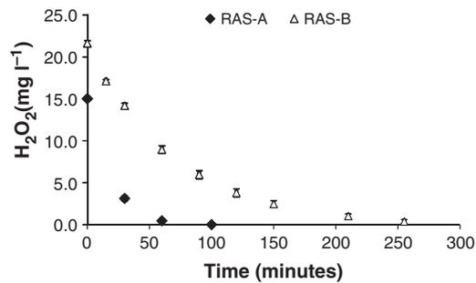
**Figure 2** Degradation of hydrogen peroxide (HP) following a single-dose HP in experiments with biofilter elements forms recirculating aquaculture systems (RAS)-A and RAS-B. Each series is the average of six biofilter tubes and the error bars represent the 95% confidence interval (not visible in RAS-A results).
