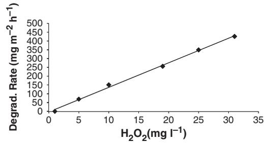
**Figure 8** Surface specific removal of hydrogen peroxide (HP) in recirculating aquaculture system-A biofilter tubes, based on linear regression analysis of the initial HP concentration ( $t = 0-15$  min) at different dosages.
