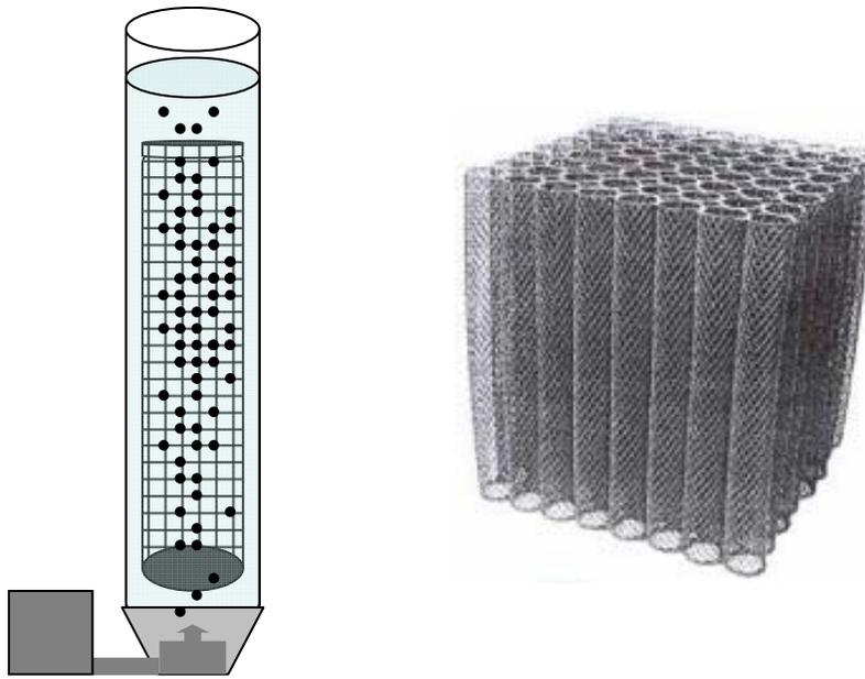
**Fig. 7.3.** Left: Illustration of a single unit of the experimental set-up to test biofilter nitrification performance. A detached Bioblok® biofilter cylinder (Ø 55mm; L 550 mm) can be submerged and provided with air by an airpump connected to a diffuser or optional internal flow from a circulation pump. Right: Bioblok 200 module; 55\*55\*55 cm; ([www.expo-net.dk](http://www.expo-net.dk)).
