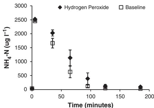
**Figure 3** Total ammonium nitrogen (TAN) concentration after a single hydrogen peroxide (HP) dose. The 'baseline' shows TAN changed in unexposed recirculating aquaculture system-A biofilter elements, whereas 'HP' shows TAN following an addition and complete degradation of 15 mg L<sup>-1</sup> of HP. The data are the average from all six reactor tubes and the error bars represent the 95% confidence interval.
