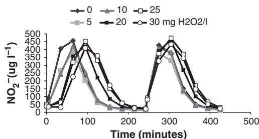
**Figure 10** Nitrite-N concentration in six biofilter tubes from recirculating aquaculture system-A after spiking with both NH<sub>4</sub>Cl and different initial hydrogen peroxide dosages. NH<sub>4</sub>Cl was respiked at  $t = 240$  min.
