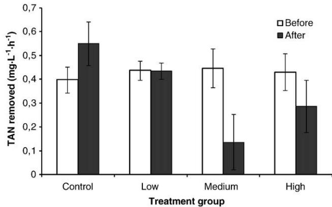
**Fig. 3.** TAN removal rate in biofilters from RAS spiked with NH<sub>4</sub>Cl before and after PA+ addition (Day -1 and Day +1). Values represent mean ± std based on linear regression of triplicate experiments of each four treatment group (N = 12).
