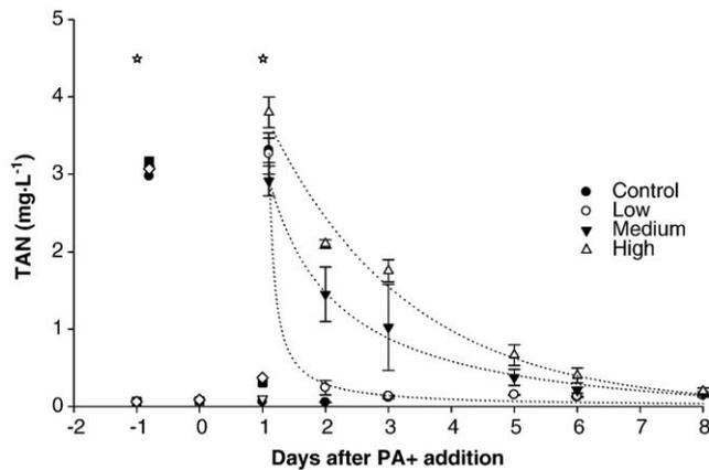
**Fig. 4.** TAN concentration in RAS before and after PA+ addition at Day 0. PA+ was added at dosages equivalent to 8, 16 and 24 ml PA+ per m<sup>3</sup> (low, medium and high, respectively). Asterisks indicate events (Day -1 and 1) where NH<sub>4</sub>Cl was added to the systems.
