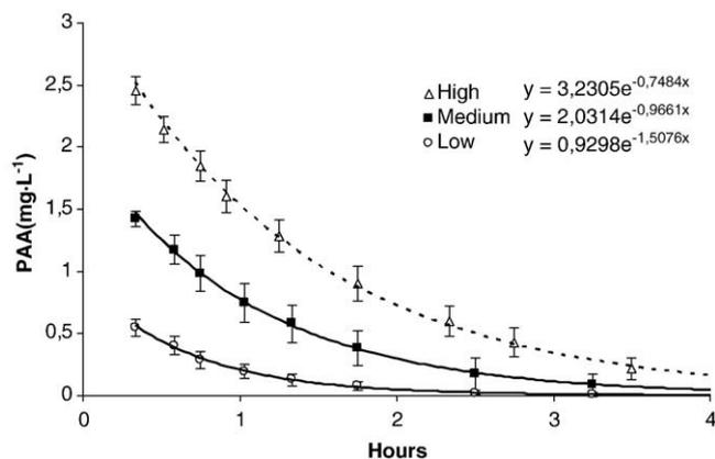
**Fig. 2.** Peracetic acid (PAA) decay after application to biofilters from RAS. Data represent PAA concentration (mean  $\pm$  std.) of triplicate experiments with low, medium and high PAA dosage, equivalent to nominal concentrations of 1.0, 2.0 and  $3.0 \text{ mg L}^{-1}$ . Exponential regression equations listed, all have  $R^2 \geq 0.995$ .
