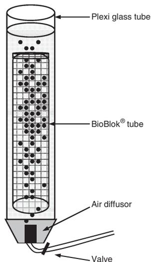
**Figure 1** The set-up for single unit experiments with BIO-BLOK<sup>®</sup> biofilter cylinder elements from different recirculating aquaculture systems.
