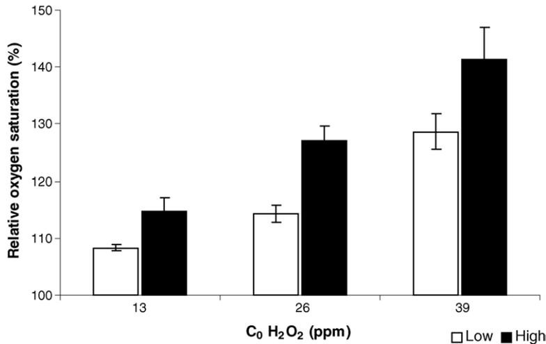
Fig. 3. Maximum oxygen concentration (%) measured in pilot system with various initial concentrations ( $C_0$ ) of hydrogen peroxide. Each application was made in triplicate to systems with low and high organic matter content ( $N = 18$ ).
