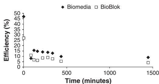
**Figure 12** Total ammonium nitrogen removal efficiency of Biomedica and BIO-BLOK<sup>®</sup> filters following multiple hydrogen peroxide (HP) additions. Initial HP application at  $t = 0$ . NH<sub>4</sub>-N degrading efficiency was calculated by (Outlet–Inlet)/Inlet.
