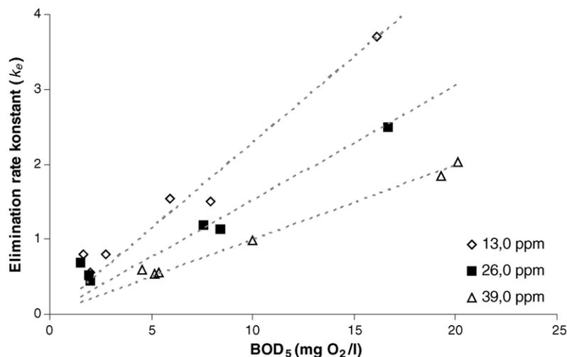
Fig. 2. Relation between elimination rate constant ( $k_e$ ) and organic matter content measured as BOD<sub>5</sub> in experiments with three different initial H<sub>2</sub>O concentrations.
