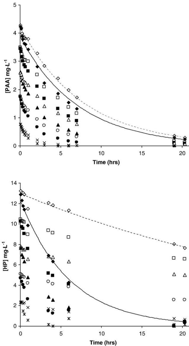
**Fig. 6.** Peracetic acid (PAA) and hydrogen peroxide (HP) decay in two types of aquaculture water with different COD levels of  $28.6 \text{ mg O}_2\text{L}^{-1}$  (open symbols, broken trend lines) and  $48.8 \text{ mg O}_2\text{L}^{-1}$  (filled symbols, solid trend lines). PA+ were added corresponding to nominal concentrations ranging from  $1.0$  to  $5.0 \text{ mg L}^{-1}$  PAA and  $2.6$  to  $13.0 \text{ mg L}^{-1}$  HP.
