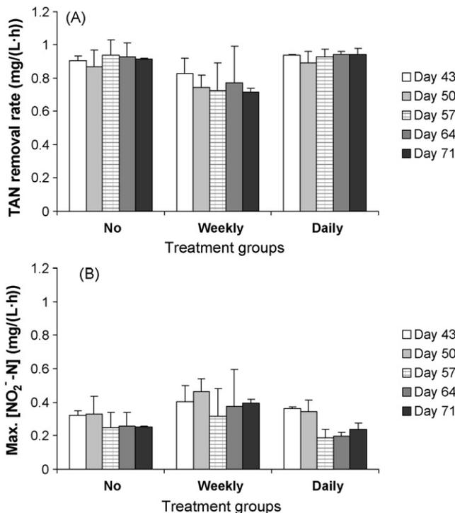
**Fig. 3.** Average ammonia removal rate (mean  $\pm$  S.D.) in 360 L pilot-scale recirculated systems over a four-week spiking period (A). Formalin was added after the control experiment, either daily, weekly or not at all. Maximal nitrite concentrations were measured concomitantly for the same three treatment groups after the ammonia spike (B).
