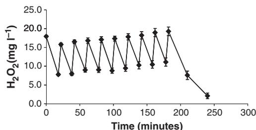
**Figure 4** The concentration of hydrogen peroxide (HP) over time in the six reactor tubes containing recirculating aquaculture system-A biofilters. The reactor tubes were spiked with HP every 20 min. The error bars represent 95% confidence interval.
