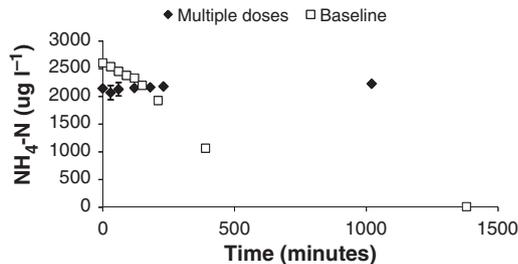
**Figure 7** Total ammonium nitrogen (TAN) concentration in recirculating aquaculture systems (RAS-B) biofilter tubes after multiple hydrogen peroxide (HP) exposure. The 'baseline' shows the TAN concentration in unexposed RAS-B biofilters, while 'multiple H<sub>2</sub>O<sub>2</sub> doses' shows the TAN concentration shortly after multiple HP doses and complete HP removal. The data are the average from all six reactor tubes and the error bars represent the 95% confidence interval.
