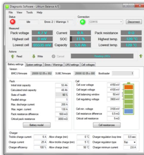
Fig. 2-6. Snapshot of ad hoc SW to manage BMS settings by Lithium Balance [42].
