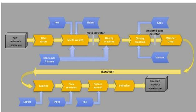
Fig. 2. Production flow of Line 1.
