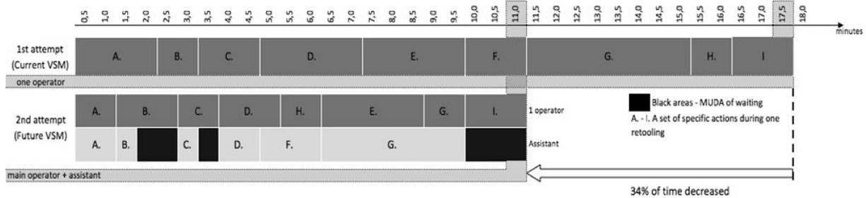
Fig. 9. Comparison of retooling time before and after the addition of helper (retooling assistant).
