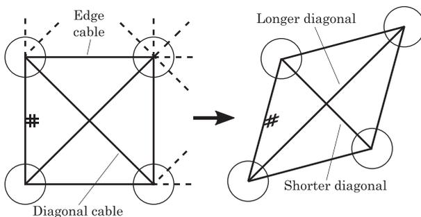
**Figure 10.** Assembly of cables into unit cells which can undergo shearing. Grippers are shown as circles but do not have any physical extent in the model. Fiber angles are indicated at the left edges.
