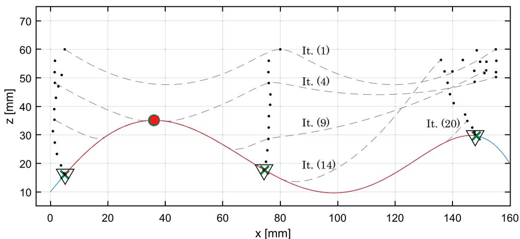
Figure 15. Draping of 2D ply onto mold with gripper trajectories generated from optimization. The gray dashed lines show the ply in iterations 1, 4, 9, 14 and 20. The red line shows the ply in the final iteration 24.
