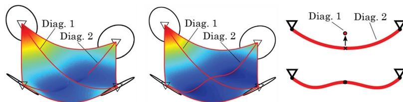
**Figure 11.** The postprocessing approach for ensuring continuity with the diagonals. Left: before postprocessing. Center: after postprocessing (diagonals are coincident). Right: 2D view of postprocessing.
