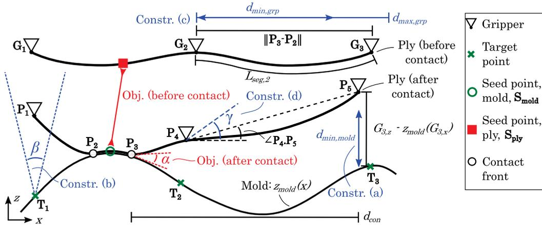
**Figure 14.** Graphical representation of objectives and constraints in optimization setup. For ease of viewing, each criterion is only shown once, but e.g. “Constr. (b)” applies for all target points.
