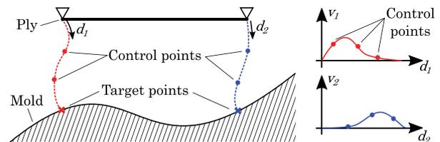
Figure 4. Possible parameterization of gripper trajectories ( $d_1$  and  $d_2$ ) and velocity profiles ( $v_1$  and  $v_2$ ) using splines.
