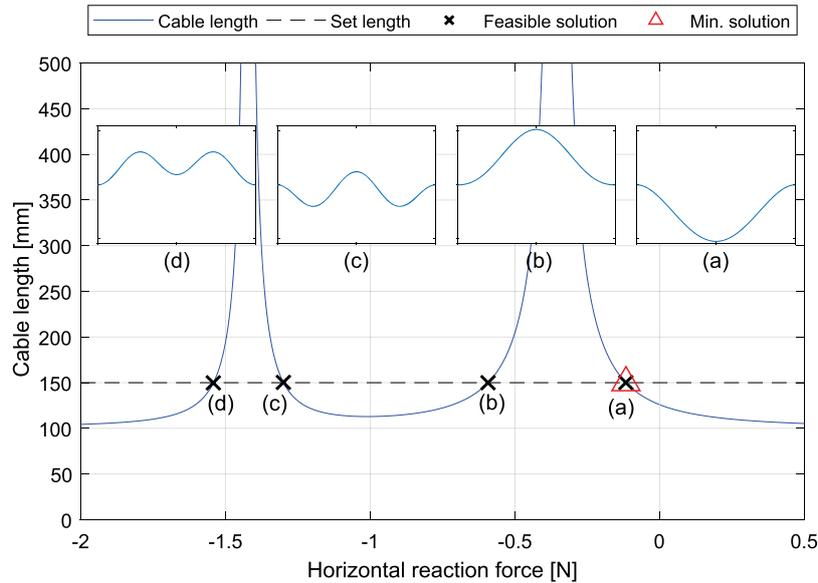
**Figure 13.** Cable length vs. horizontal reaction force for cable with 100 mm span and fixed end point rotations. Four values of the reaction force yield the sought length of 150 mm. The peaks located at -0.355 N and -1.42 N correspond to the singularities in the differential equation.
