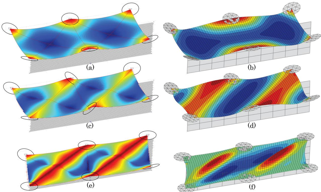
**Figure 16.** Draping onto flat parallelogram mold with cable model ((a), (c) and (e)) and FE model ((b), (d) and (f)). The rows correspond to the initial configuration, 10% done and 75% done respectively.
