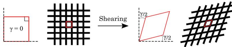
**Figure 2.** Fabric shear involving fiber tows rotating at the cross-over points.  $\gamma$  is the shear angle.
