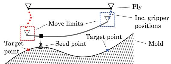
Figure 5. Parameterization using incremental optimization with inspiration from manual layup.
