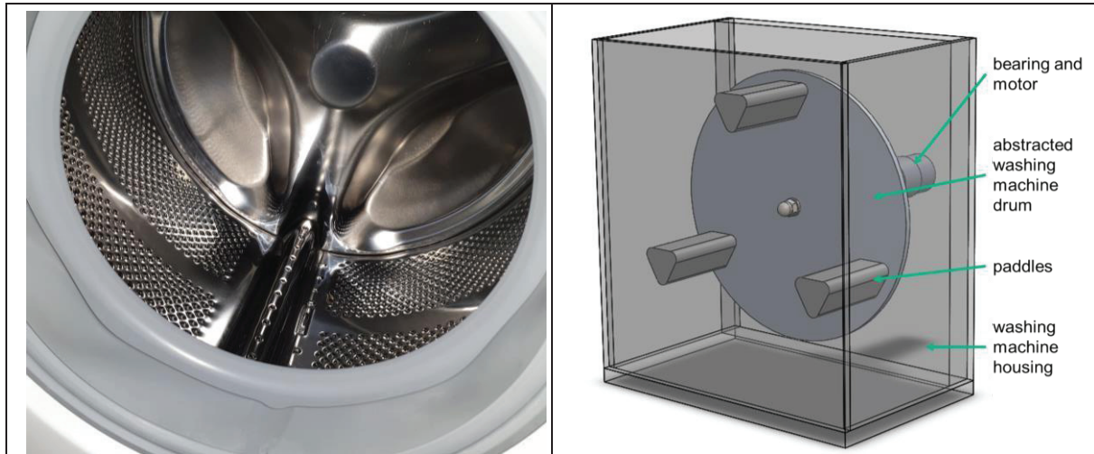
Fig. 3: Washing machine paddle inside a washing machine drum (l.) and washing machine test bench for investigation purposes (r.)
