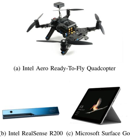
Fig. 1. Hardware setup used for the proposed framework
