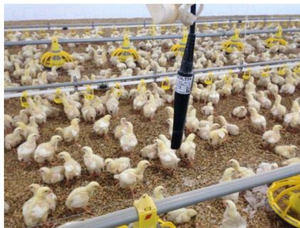
**Figure 1.6:** Combined temperature and humidity sensor.
