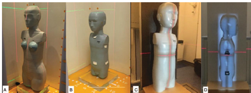
Figure 1. (A), Female phantom (representing an adolescent) in the EOS stereo-radiography scanner. Anterior-posterior-lateral (APL) position (frontal and lateral images are acquired simultaneously). (B), Child phantom (representing a 5-year-old) in EOS scanner in APL position. (C,D), Child phantom in the conventional digital radiology system in AP and lateral position (frontal and lateral images are acquired independently).
