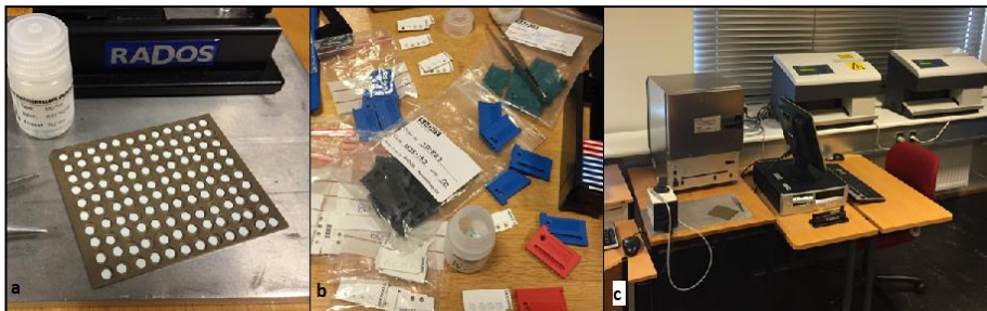
Figure 8, (a) TLDs, (b) cassettes and magazine, (c) from left; annealing oven (TLDO. PTW, Freiburg Germany), irradiator (IR-2000) and reader (Re-2000)
