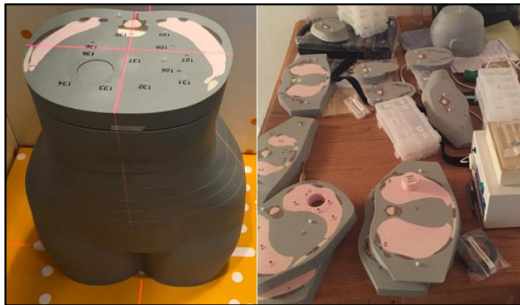
Figure 5, the adult female phantom in the scanner and disassembled, illustrating examples of different phantom slices and placement of inner organs.
