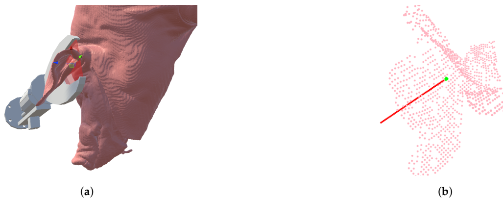
Figure 1. (a) Correct tool pose illustrated using 3D models of the tool and pig. (b) A point cloud of the ear region with our representation of a 5-DoF cutting plane consisting of P_0 (green) and \vec{n}\hat{z} (red).
