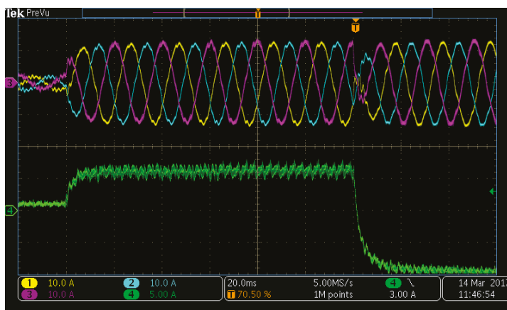
Figure 18. Experimental results of the HFLMC operating in charger and inverter mode: grid currents ( i_{ga} , i_{gb} , i_{gc} ) [yellow, blue, magenta] and battery current ( i_{DC} ) [green].
