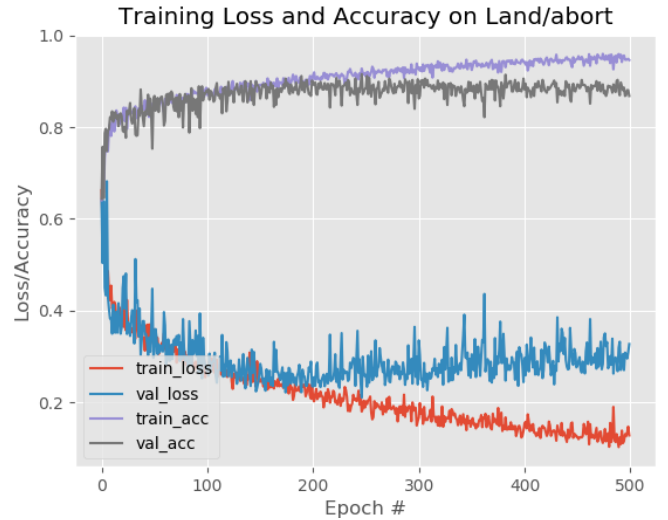
Fig. 7: Illustration of the learning curves for the LeNet classifier with a dropout layer.
