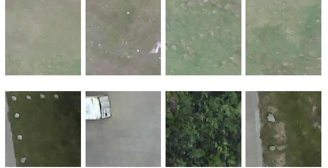
Fig. 5: Frames showing examples of (top row) "landing locations", and (bottom row) "not landing locations".
