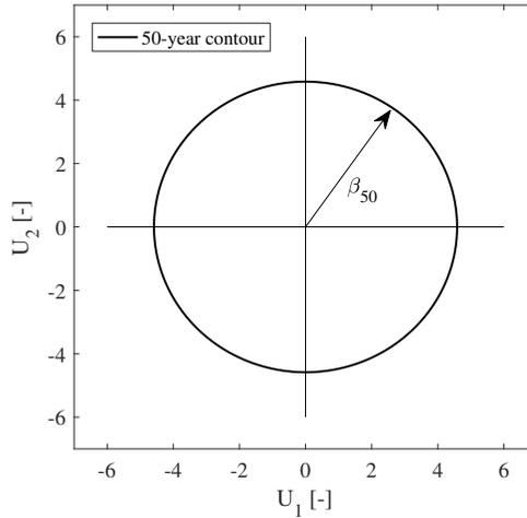
Fig. 4.3: Illustration of U-space for  $\beta_{50} = 4.58$  (Velarde, Vanem, et al., 2019)
