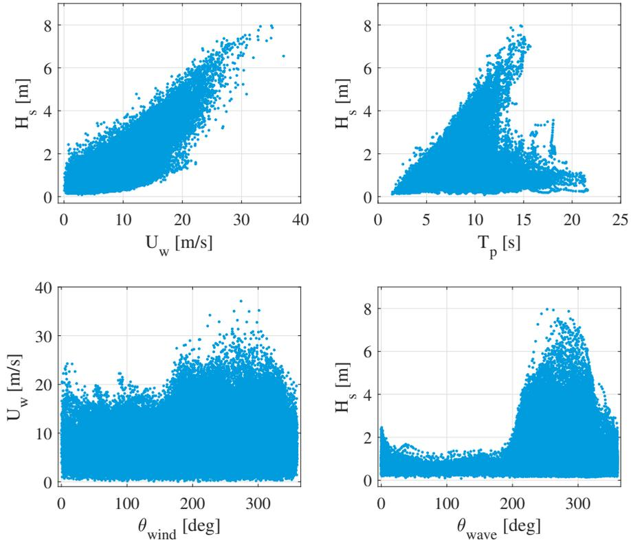
**Fig. 3.2:** Illustration of necessary metocean data for fatigue assessment of OWTs. Hindcast data is from *Vesterhav Nord* OWF.
