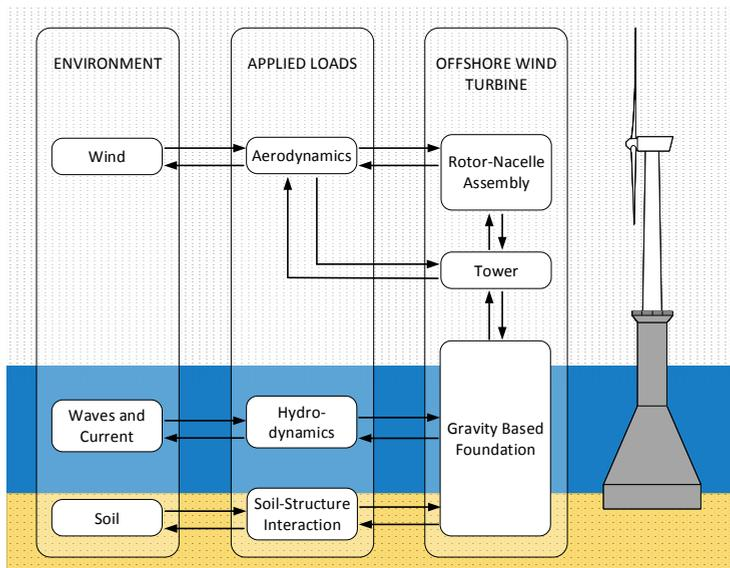
**Fig. 2.1:** Interaction between wind loads, wave loads, soil and an offshore wind turbine (Velarde, Kramhøft, & Sørensen, 2019a)
