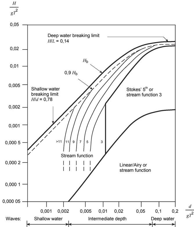
Fig. 2.2: Selection of suitable wave theory as a function of normalized water depth ( $d/gT^2$ ) and normalized wave height ( $H/gT^2$ ) (International Electrotechnical Commission, 2009)
