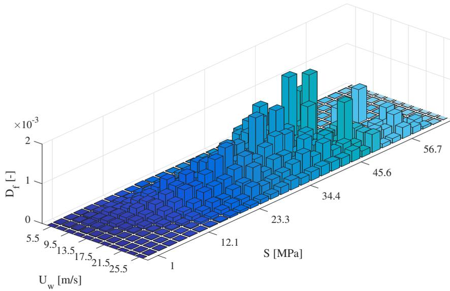
**Fig. 3.8:** Estimated fatigue damage as a function of mean wind speed at hub height ( $U_{hub}$ ) and stress range ( $S$ ) for an operating 10 MW offshore wind turbine supported by a monopile
