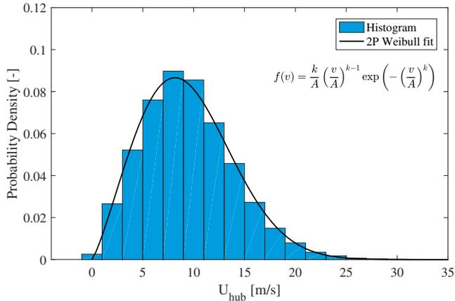
**Fig. 3.3:** Wind speed ( $v$ ) distribution and Weibull fit ( $A = 10.67 \text{ m/s}$ ,  $k = 2.23$ ) using hindcast data from *Vesterhav Nord* OWF. Adapted from Velarde et al. (2019).
