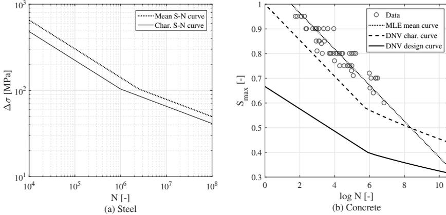
**Fig. 3.7:** S-N curves for (a) steel and (b) concrete based on DNV GL (2016a; 2018a) standards. Adapted from Velarde, Kramhøft, Sørensen, and Zorzi (2019) and Velarde, Mankar, et al. (2019), respectively.
