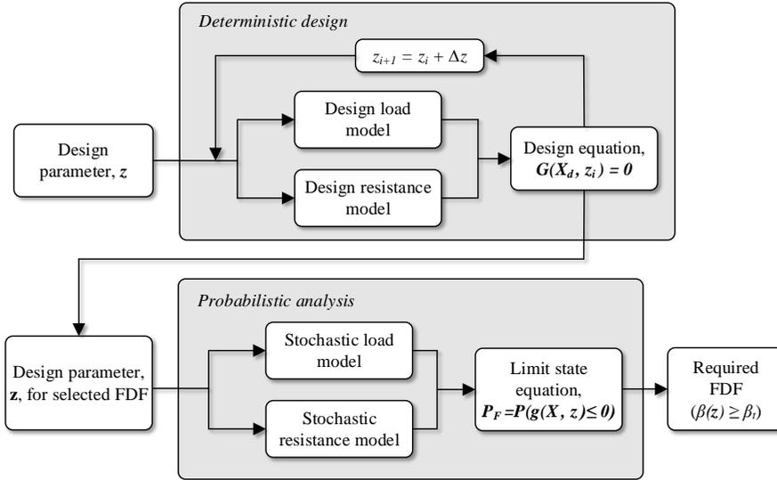
**Fig. 4.7:** Reliability-based approach for calibration of material partial safety factor, ( $\gamma_m$ ) and fatigue design factors (FDFs). Adapted from Velarde, Mankar, et al. (2019).
