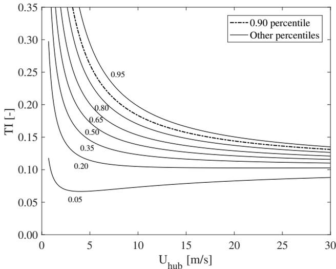
**Fig. 4.2:** Turbulence intensity (TI) distribution and design value (0.90 percentile) based on IEC 61400-1 (2005)
