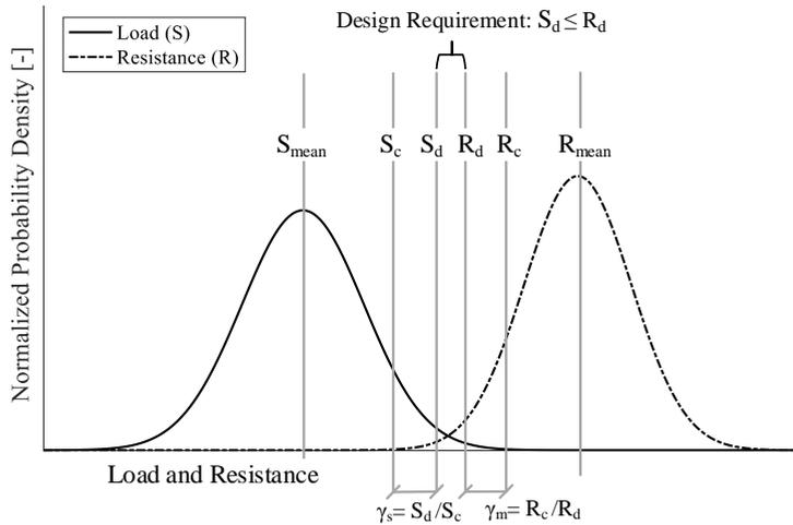
Fig. 4.6: Design principle based on load and resistance factor design (LRFD)
