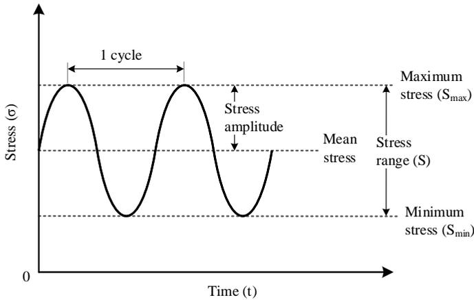
Fig. 3.6: Stress cycle definitions considering a constant amplitude stress history
