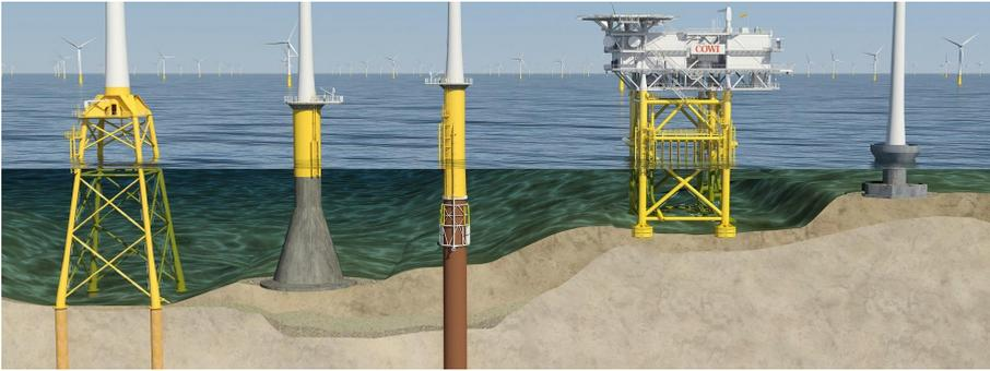
Fig. 1.1: General types of bottom-fixed OWT foundations © COWI
