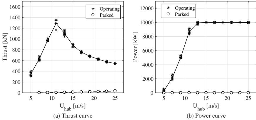
**Fig. 3.4:** Derived (a) thrust and (b) power curve based on time-domain simulations of DLC 1.2 for the DTU 10 MW reference OWT with six realizations per wind speed. Adapted from Velarde et al. (2019).
