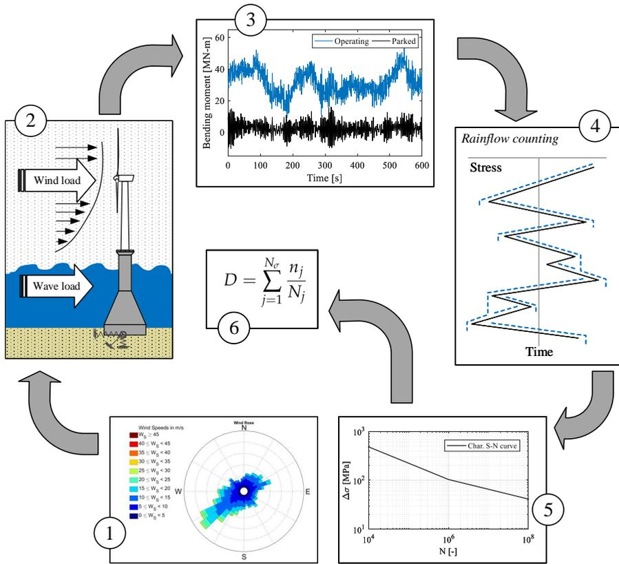
**Fig. 3.1:** Procedure for fatigue design of OWT substructures based on S-N approach
