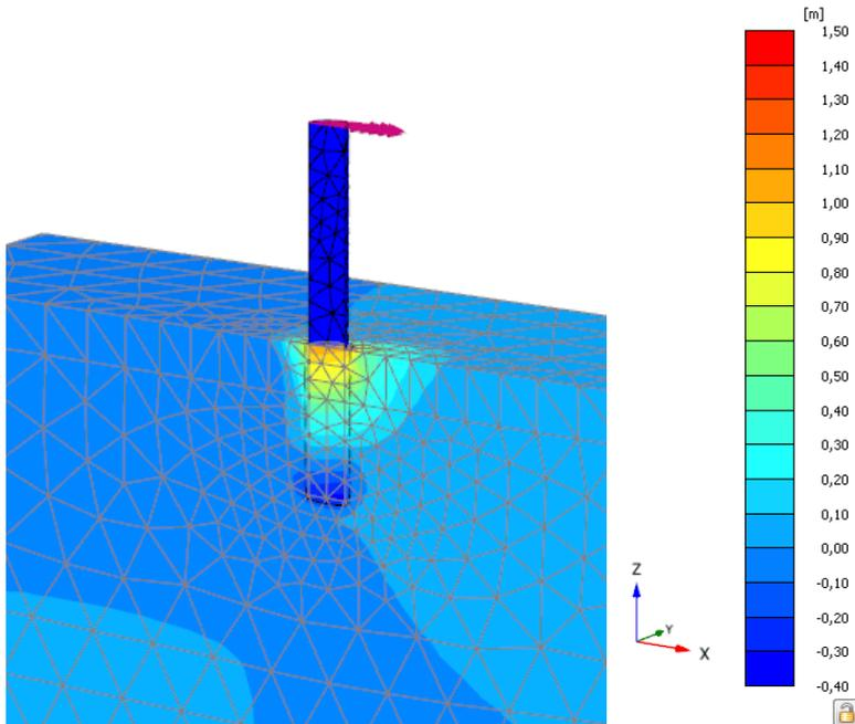
**Fig. 2.4:** Finite element modeling of soil-structure interaction in PLAXIS 3D. Adapted from Velarde et al. (2019).
