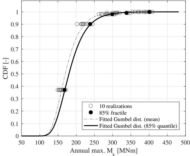
**Fig. 4.5:** Illustration of extreme response distribution at GBF ring beam section. Gumbel distribution is fitted to 0.85 fractile with mean value,  $E[M_x] = 187.7 \text{ MNm}$  and standard deviation,  $\sigma_{M_x} = 40.4 \text{ MNm}$ . Adapted from Velarde, Kramhøft, and Sørensen (2019b).
