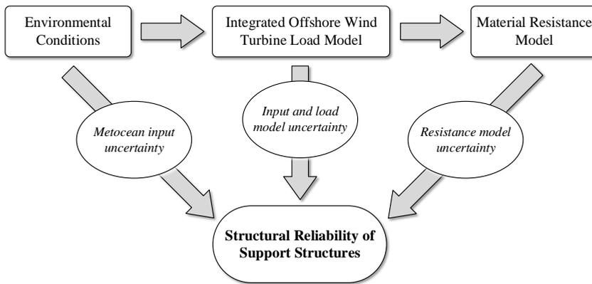
**Fig. 1.2:** Primary sources of uncertainties in reliability assessment of offshore wind turbine support structures
