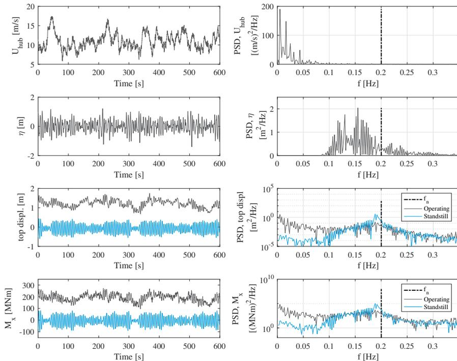
**Fig. 3.5:** Time domain simulation and frequency domain signals of OWT response and selected environmental condition ( $U_{hub} = 11$  m/s,  $TI = 0.18$ ,  $H_s = 1.55$  m,  $T_p = 7.4$  s,  $\gamma_{wave} = 1.0$ ). The natural frequency ( $f_n$ ) of the 10 MW OWT is also illustrated.
