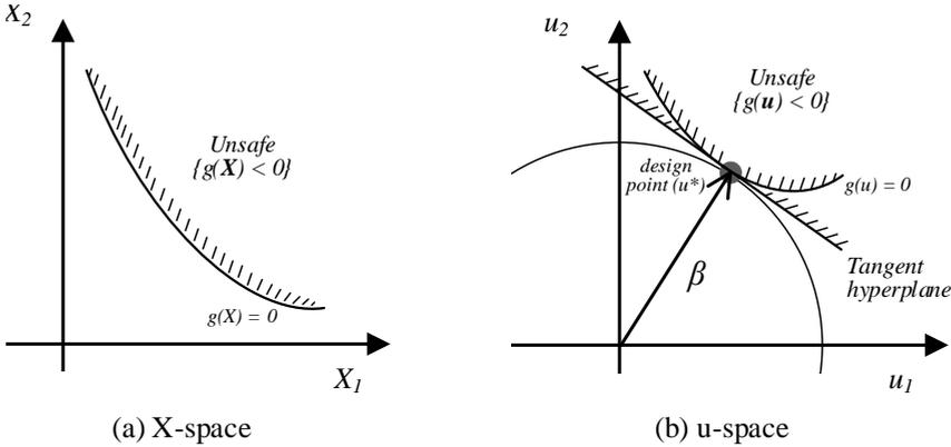
Fig. 4.1: Graphical illustration of failure surfaces in (a)  $X$ -space and (b)  $u$ -space
