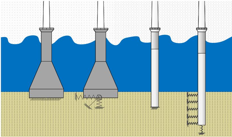
**Fig. 2.3:** Typical representations of soil-structure interaction in integrated aeroelastic models. From left to right: fixed base, coupled springs, apparent fixity model, distributed springs.
