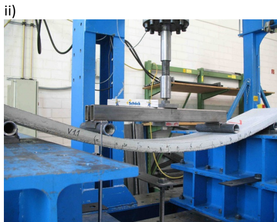
i) Example of FRP reinforcement used in real life concrete structures, ii) Deflected concrete beam with internal GFRP reinforcement.
