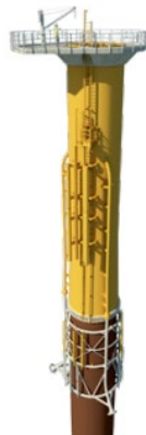
Sketch drawing of a monopile.
