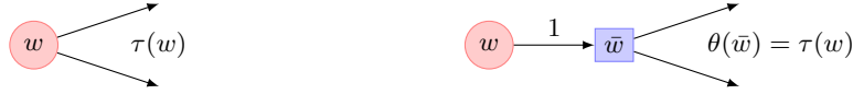
Fig. 3. (Left) A state in the original MC \mathcal{M} ; (Right) The MC \bar{\mathcal{M}} constructed from \mathcal{M} . In \bar{\mathcal{M}} , each state w \in S moves to its counterpart \bar{w} \in \bar{S} that proceeds as w does in \mathcal{M} .
