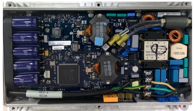
Fig. 3. Photo of the Enphase microinverter M250 [10].
