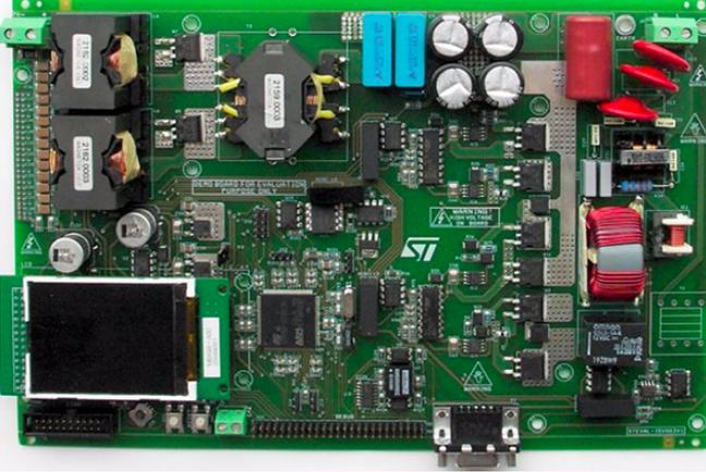
Fig. 7. Photo of the microinverter from ST Microelectronics [15].
