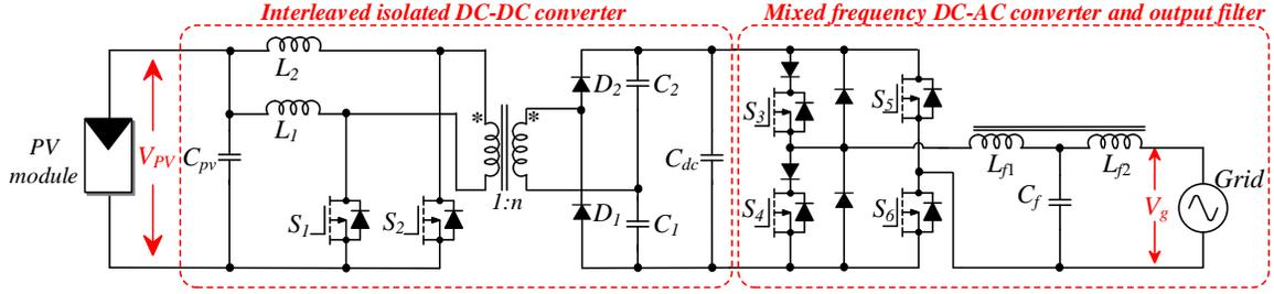
Fig. 6. The microinverter topology from ST Microelectronics [15].
