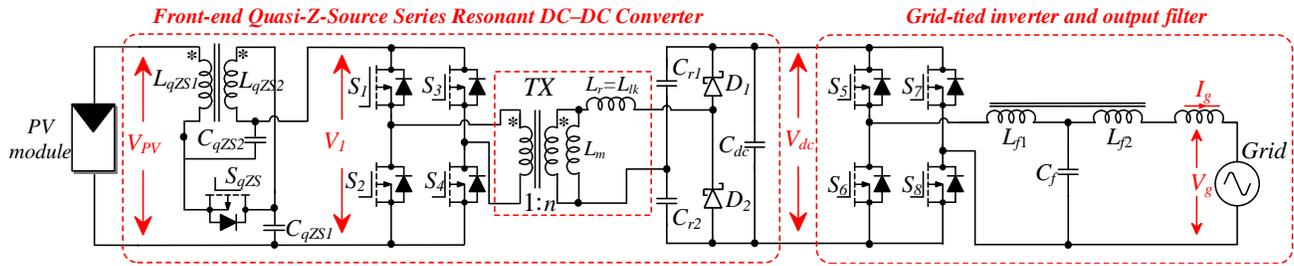
Fig. 8. Impedance-source-based PV microinverter topology [24].
