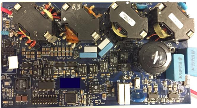
Fig. 9. Photo of the impedance-source-based PV microinverter topology [24].
