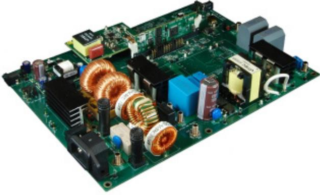
Fig. 5. Photo of TI's microinverter [21].
