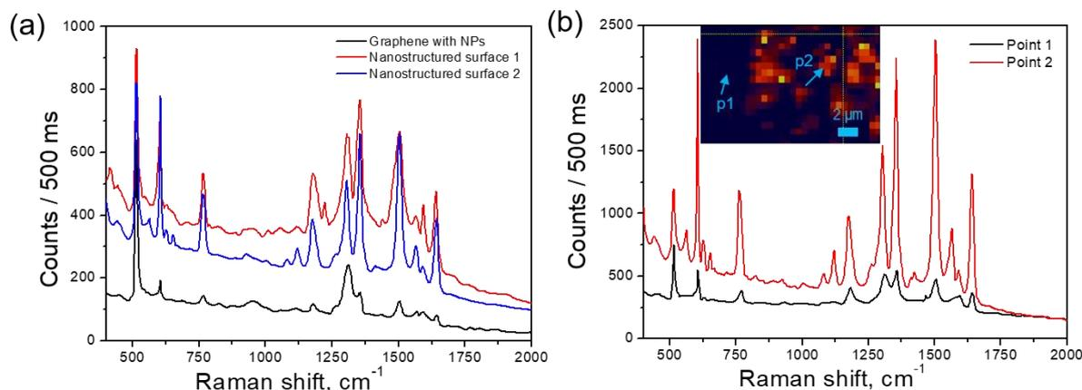
**Figure 2.** a) Average Raman spectra obtained from continuous and nanostructured graphene with NPs, b) Raman spectra from the points indicated by the arrows in the inserted figure. P1 – point out of array, P2 – hot spot from the array.
