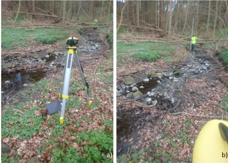
Figure 2.7: Illustration of the equipment for measuring the cross-sections of Polsterbæk. a) shows the electronical levelling device, and b) shows the post used to register the vertical variations in the stream.
