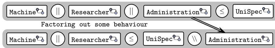
Fig. 6. One possible step in Stepwise modularisation of requirements: Factoring out the behaviour of the Administration.
