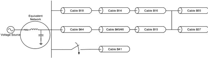
Fig. 10. Single line diagram of the simulated network
