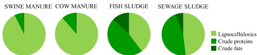
Figure 24: Composition of swine manure, cow manure, fish sludge, and sewage sludge in terms of lignocellulosics, crude proteins, and crude fats (data from Table 1 in [C]).
