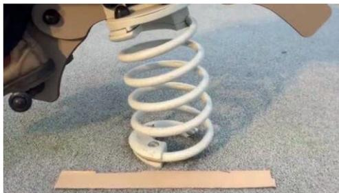
Figure 10: Students measuring the deflection of the spring
