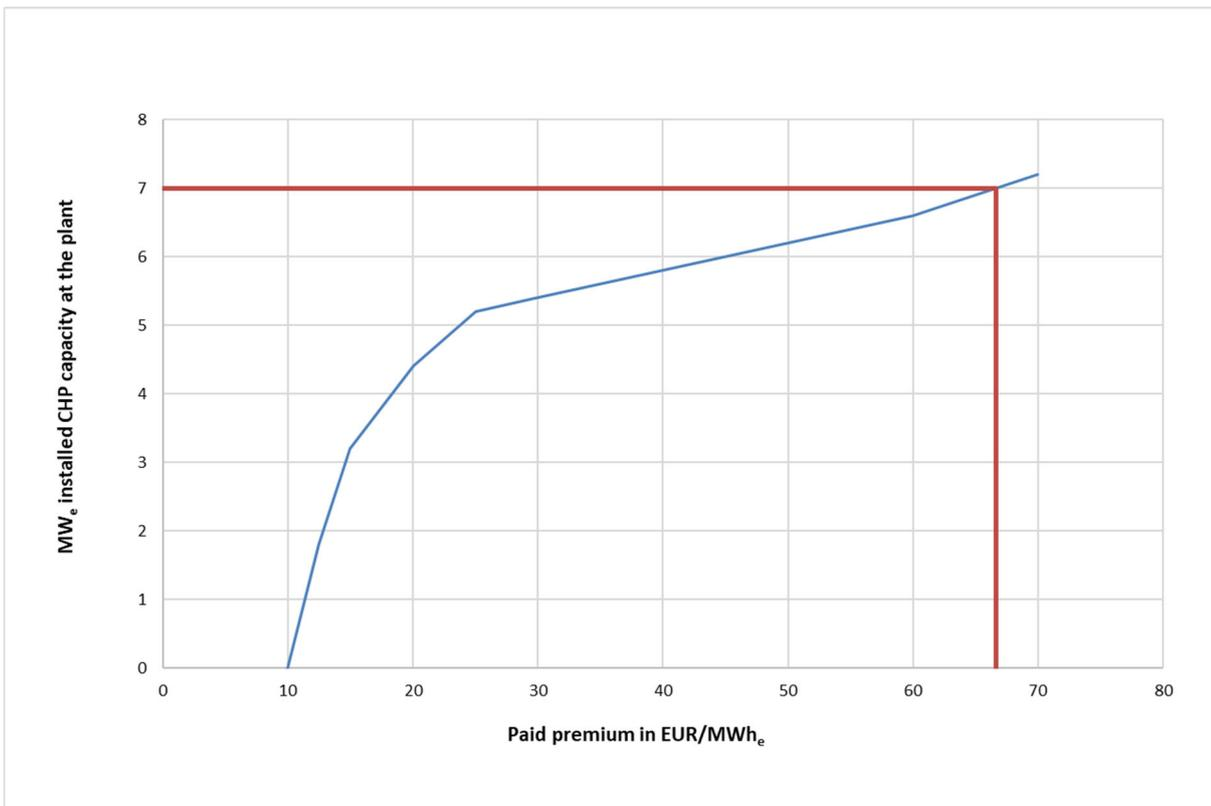
Figure 5: Determining the paid premium resulting in a total CHP capacity of 7 MW<sub>e</sub> being equal to 66.67 EUR/MWh<sub>e</sub>.
