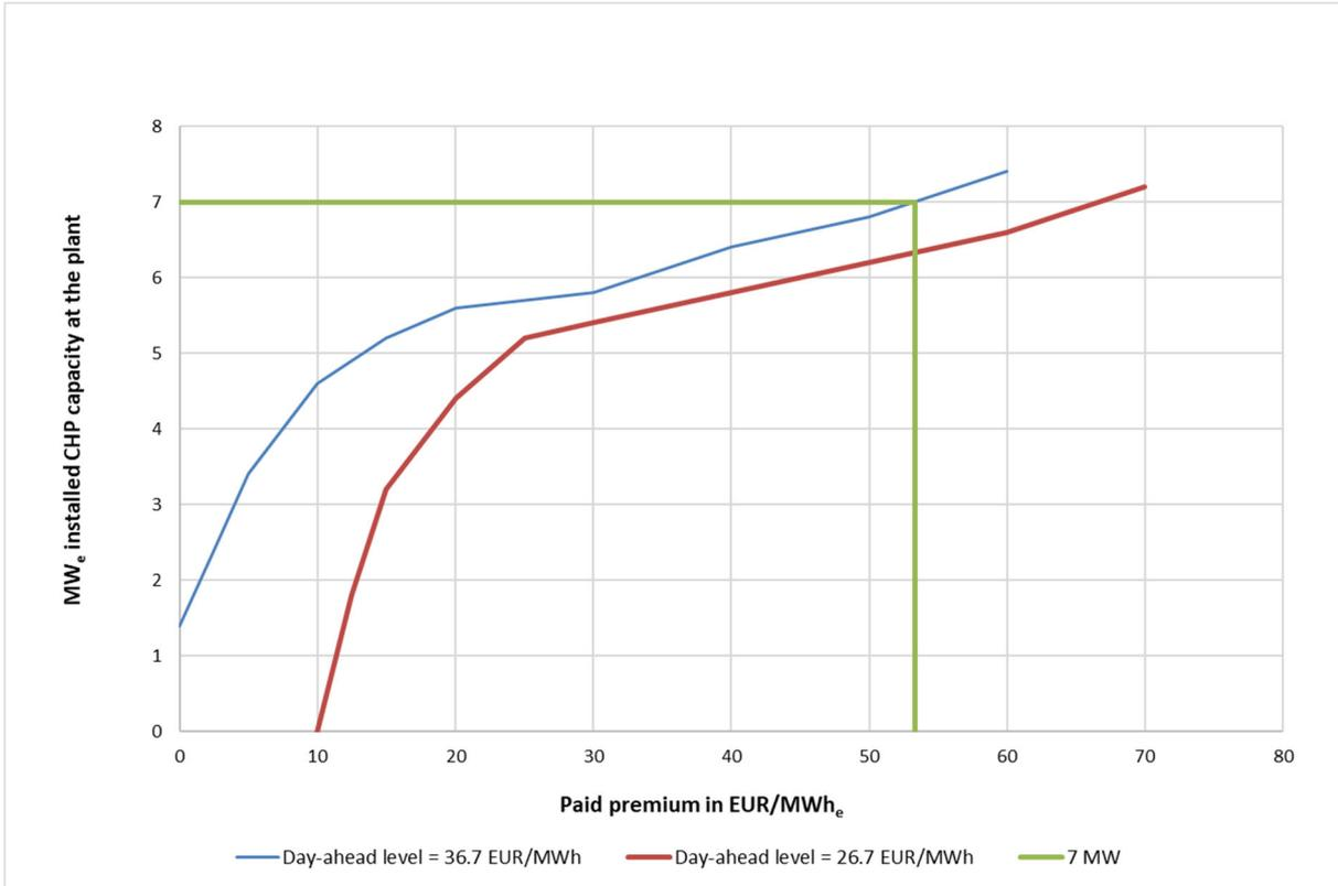
Figure 6: Determining the paid premium resulting in the same total CHP capacity of 7 MW<sub>e</sub> being equal to 53.33 EUR/MWh<sub>e</sub> when the day-ahead level is 36.7 EUR/MWh<sub>e</sub>.
