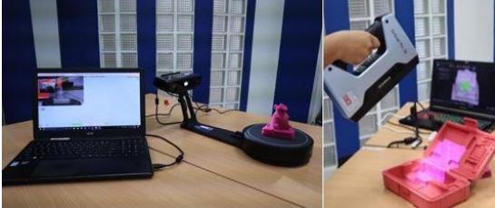
Figure 2. 3D scanning and exporting STL files
