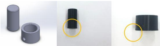
Figure 4. CAD design and testing shrinkage effect
