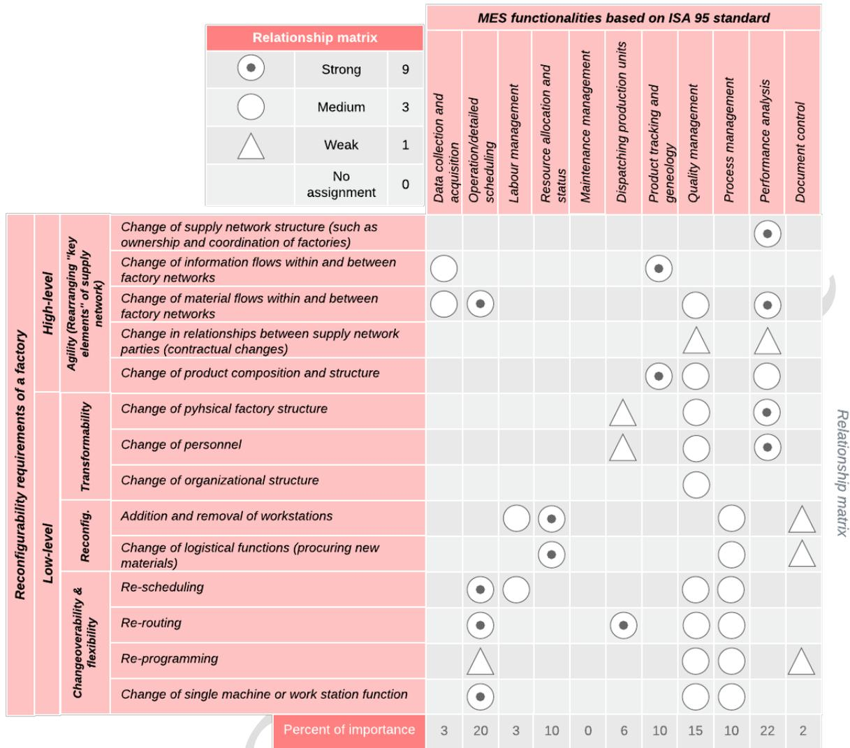
Fig. 4. House of quality (QFD) matrix - Linking reconfigurability requirements and MES functionalities.
