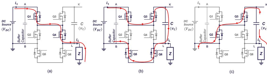
Fig. 1: Single PN cell operation in (a) P-state, (b) 0-state, and (c) N state
