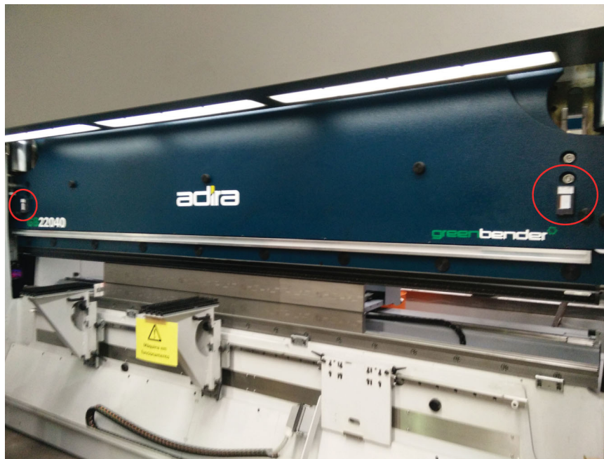
Figure 6. Frontal view of the machine with two Inertial Measurement Units (IMUs).
