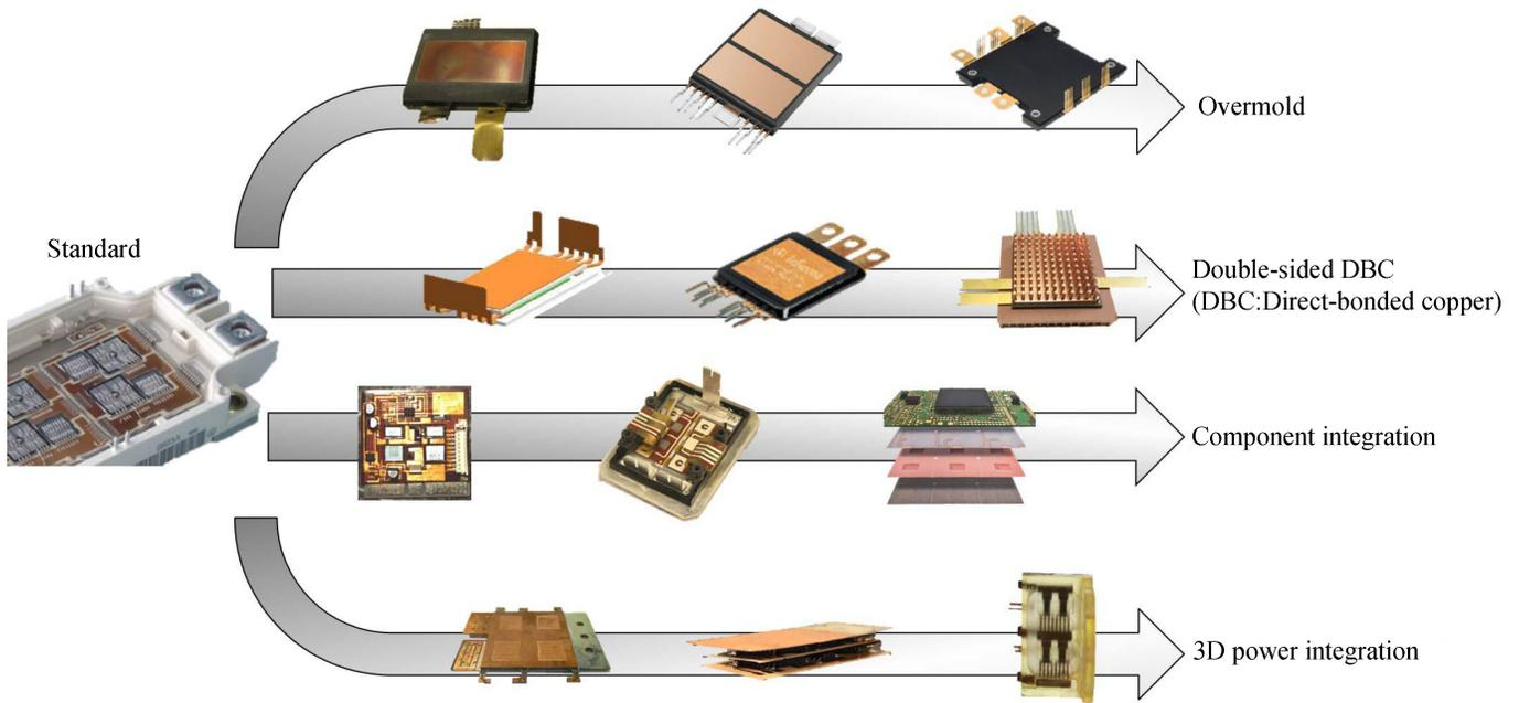
Fig. 6. Advances in packaging elements for power modules [18].
