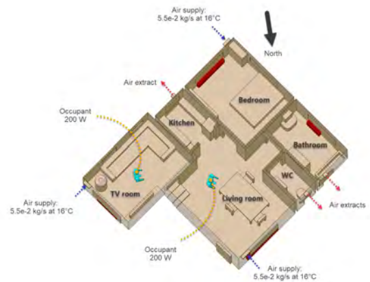
Figure 7: Simulation setup for the first-floor apartment
