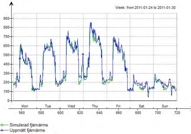
Figure 7: Delivered district heating profile kW, Measured (Blue) vs Simulated (Red), a week in February
