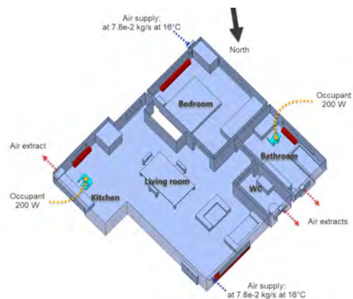
Figure 8: Simulation setup for the second-floor apartment
