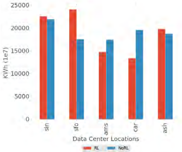
Figure 4: Total Site annual energy for statically (NoRL) configured IT load and dynamically reset (RL) IT loads.
