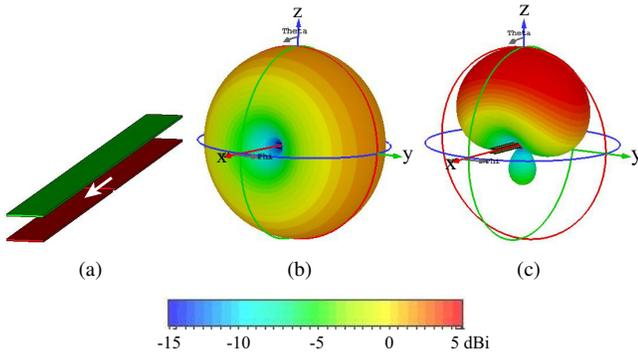
Fig. 3. Quasi-Yagi system. (a) Simulation model of the two parallel elements, one driven (red) and one parasitic element (green). Directivity pattern for the element lengths: (b)  $\ll \lambda/2$ , and (c)  $\sim \lambda/2$ .
