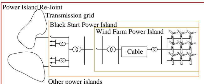
Fig. 1. Stages of the black start procedure implemented by an offshore wind farm.
