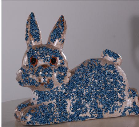
**Fig. G.5:** An image used as input to the SfM solution and calculated feature points. A radius is set around each of the features and all points that are in the area are projected to the reconstructed mesh
