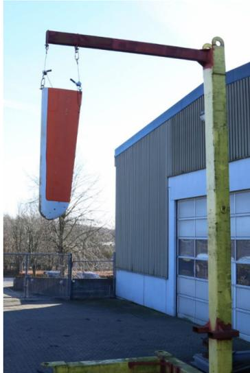
**Fig. D.2:** The wind turbine segment used for the research in the paper, mounted horizontally on a gantry. The blade can sway in the wind unobstructed, for a more realistic image capture setup.
