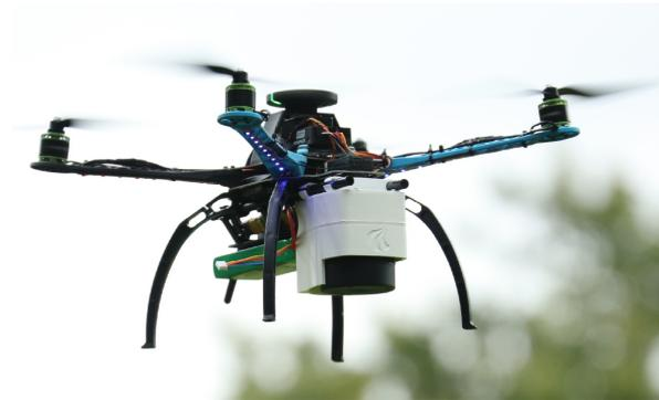
Fig. 2.10: Initial testing drone - the Iris+, together with its sensor payload
