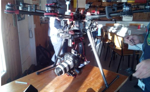
**Fig. 2.11:** The second testing drone - DJI S1000, used for initial experiments containing both the capturing camera and the GPS and distance sensors
