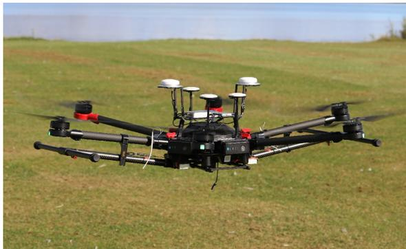
**Fig. 2.12:** The final UAV platform - the DJI Matrice 600, which was used for the real life image capturing and sensor test and as part of [50]
