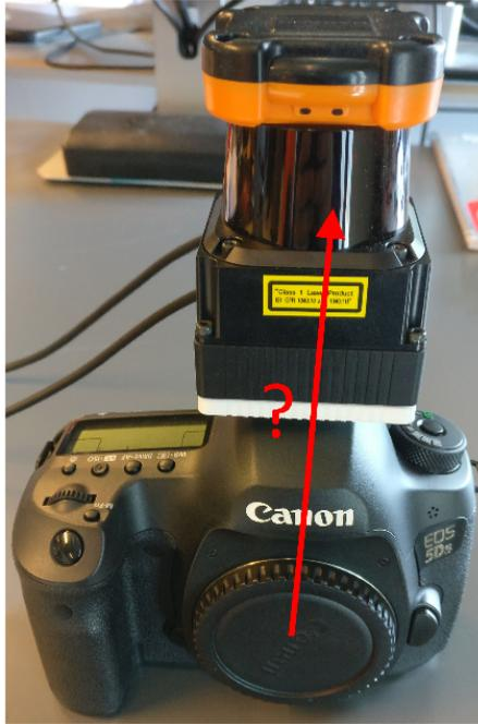
**Fig. 2.18:** The LiDAR sensor connected to the DSLR camera used for capturing the testing data [50], paper E
