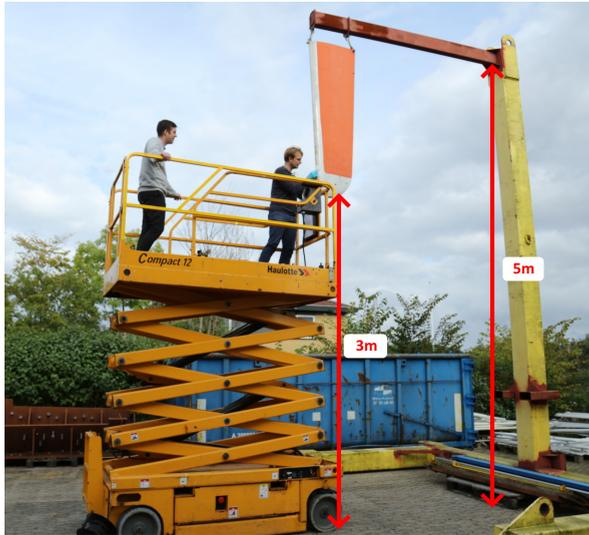
**Fig. H.1:** The wind turbine blade segment positioned on the built gantry, together with the scissor lift used for capturing image and replica data.
