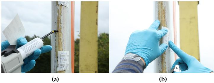
**Fig. H.4:** Replication of an area on the blade mock-up. Figure H.4a illustrates the application of the combined polymer and curing agent from a static-mixing nozzle. Figure H.4b shows the backing paper being attached by applying a gentle force to the replication material.
