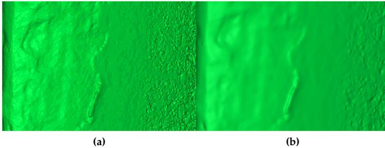
**Fig. 3.1:** Reconstructed mesh surface before (Figure 3.1a) and after (Figure 3.1b) a global smoothing algorithm is applied to remove the noisy parts. It can be seen how much of the real roughness is removed in the process
