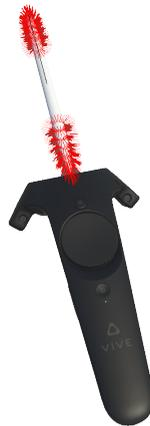
**Fig. I.1:** Rendering of our virtual VR stylus connected to the VR controller. The virtual stylus is used to virtually "touch" objects. The stylus is only seen in VR and does not exist on the real controller. The red rays cast from the stylus are shown for easier explanation of method and are not visible, when using the application.
