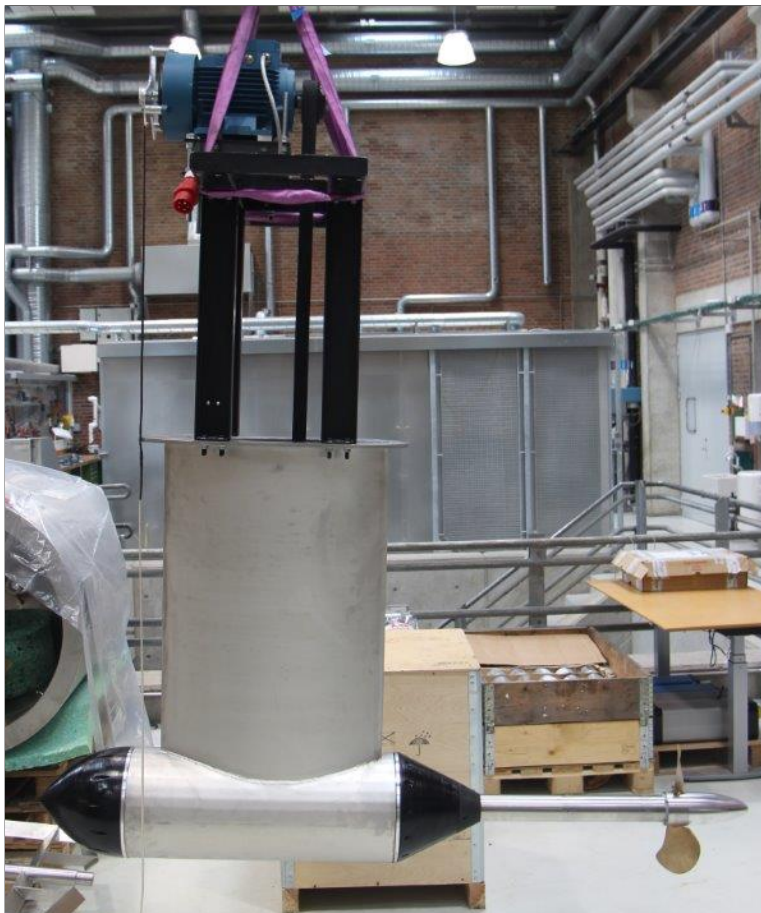
Figure 4.15: The build open-water carriage and propeller dynamometer.
