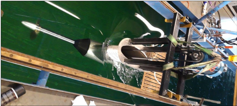
Figure 4.20: open-water carriage mounted on the towing tank carriage.
