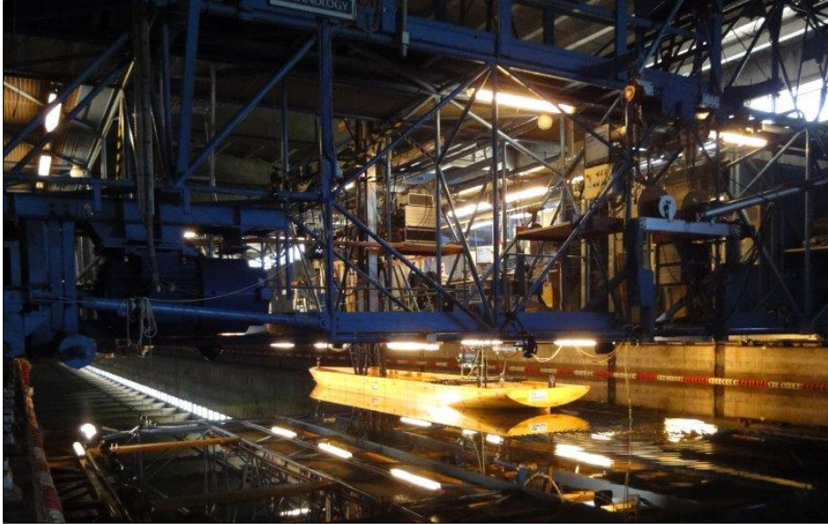
Figure 4.24: Setup for the self-propulsion tests.
