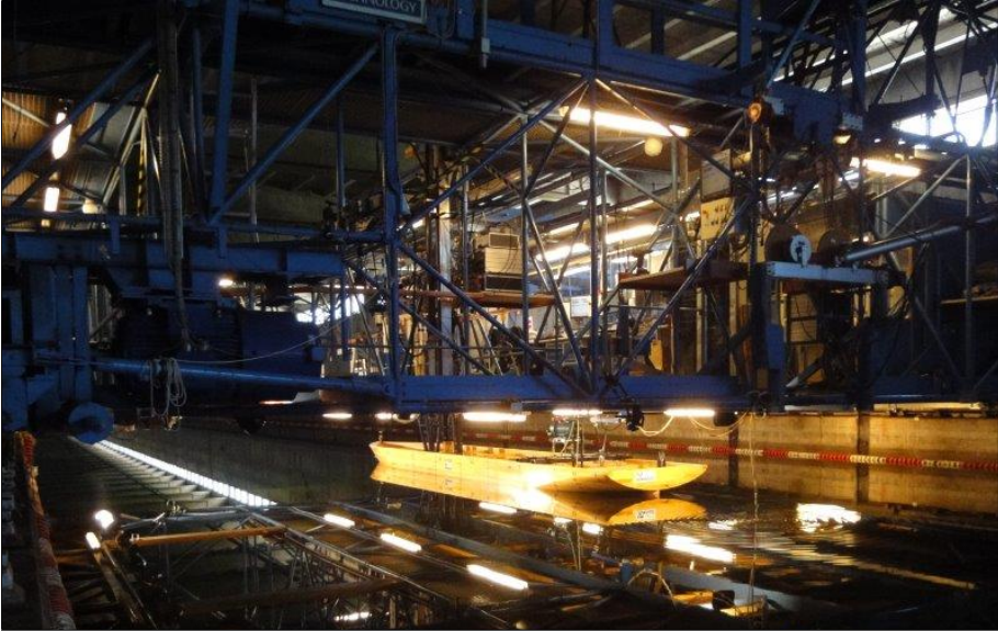
Figure 4.24: Setup for the self-propulsion tests.
