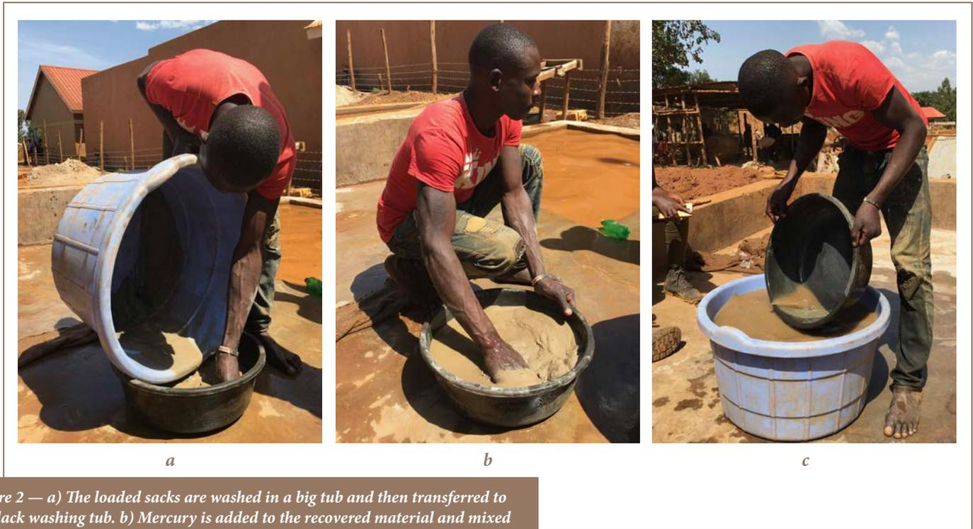
Figure 2 — a) The loaded sacks are washed in a big tub and then transferred to the black washing tub. b) Mercury is added to the recovered material and mixed by hand. c) The light minerals are discarded by gravity (washing technique) little by little until only the amalgam is left. All images published with permission.
