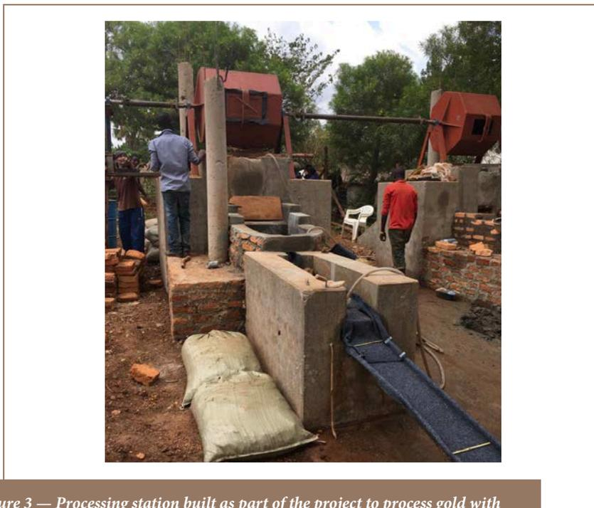
Figure 3 — Processing station built as part of the project to process gold with direct smelting. Two interconnected ball mills followed by two successive sluice boxes and a launder. Published with permission.
