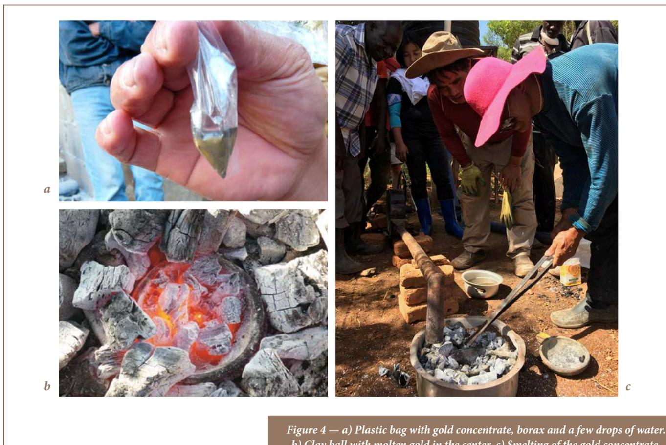
Figure 4 — a) Plastic bag with gold concentrate, borax and a few drops of water. b) Clay ball with molten gold in the center. c) Smelting of the gold concentrate. Published with permission.
