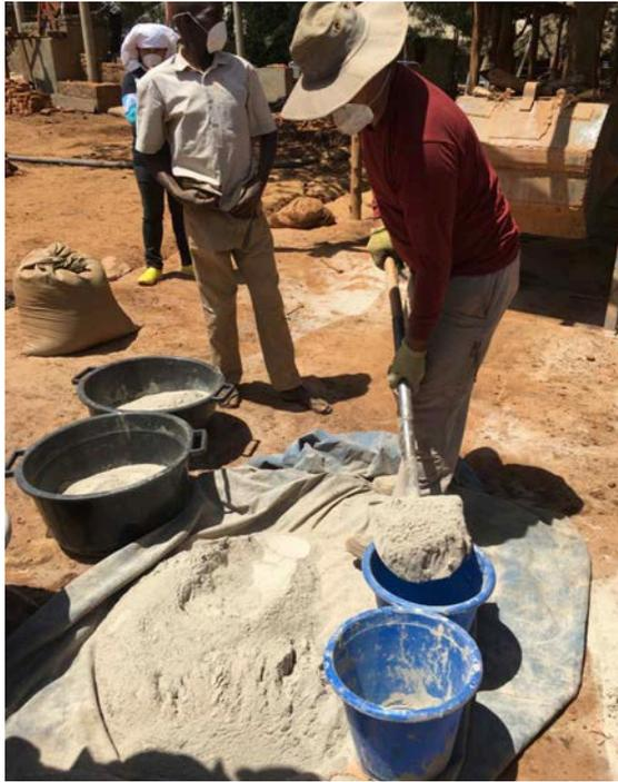
Figure 5 — The dry milled ore is divided spade by spade into two lots.
