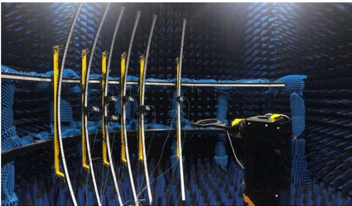
Figure 1.17: FR2 3D MPAC anechoic chamber in labs
