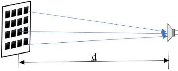
Figure 1.6: Antenna array measurement in mid-field (Fig. 1 in [41]).
