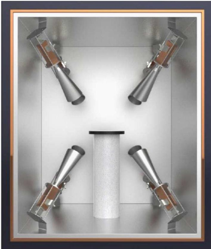
Figure 1.15: FR1 RTS anechoic chamber.
