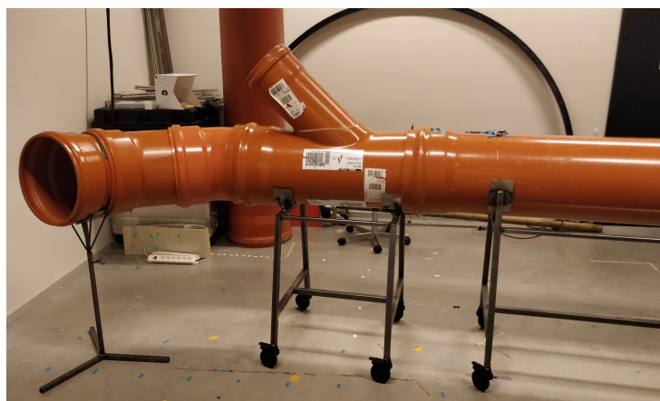
(a) View of the bigger setup consisting of a single branch pipe and bends.
