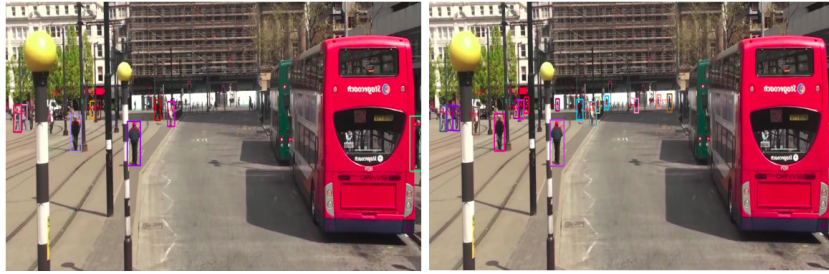
Fig. 6. left: results obtained from implicit attention-based tracker, right: results obtained via our explicit attention-based tracker. Small objects at the back are detected accurately using explicit attention (right), which are missing in left image.
