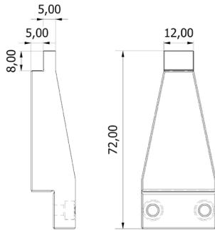
Fig. 8. Dimensions and design of the gripper.
