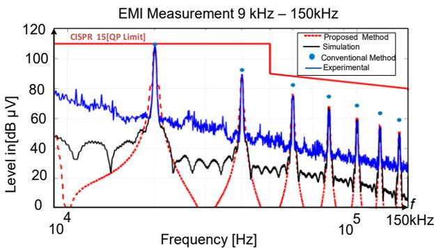
Fig. 17. Obtained DM noise results for the single-phase boost PFC with  $f_{sw} = 20$  kHz including one-stage DM EMI filter, based on proposed (32) and conventional analytical (38) approaches, simulation-based PLECS software and experimental measurement.
