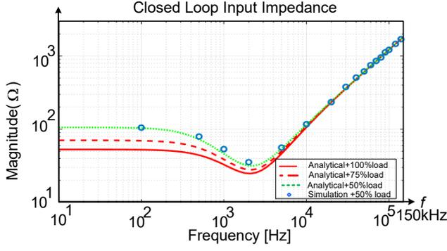
Fig. 11. Effect of output power level on close loop impedance behavior based on model from (15), and simulation using PLECS software with 50% of load. All scenarios are with low pass filter.
