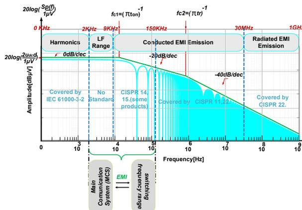
Fig. 1. Overview of the classified EMI frequency ranges according to IEC with corresponding trapezoidal waveform frequency spectra, ( $U_{dc} = 400$ ,  $f_s = 20$  kHz,  $t_r = t_f = 400$  ns,  $d = 0.5$ ).
