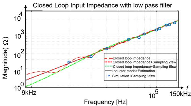
Fig. 8. Closed-loop impedance behavior based on simplified boost inductor model given by (15), the developed model in (17) with sampling  $2f_{sw}$  and  $5f_{sw}$  and simulation using PLECS software with  $2f_{sw}$  sampling. All scenarios are with a low pass filter.
