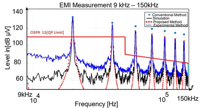
Fig. 16. Obtained DM noise for the single-phase boost PFC with  $f_{sw} = 20$  kHz without EMI filter, based on proposed (32) and conventional (38) approaches, including PLECS simulation and experimental results.
