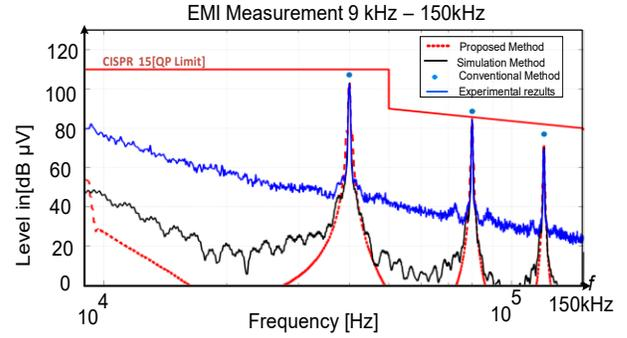
Fig. 18. Obtained DM noise results for the single-phase boost PFC with  $f_{sw} = 40$  kHz including one-stage DM EMI filter, based on proposed (32) and conventional analytical (38) approaches, simulation-based PLECS software and experimental measurement.
