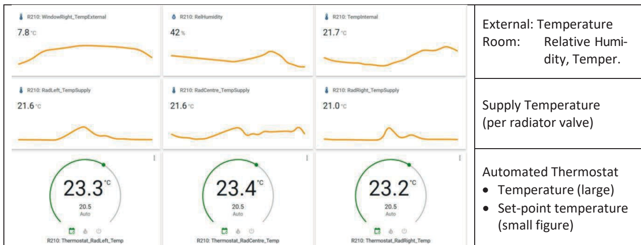
Figure 5: Initial screenshot from the BAC-system's monitoring dashboard
