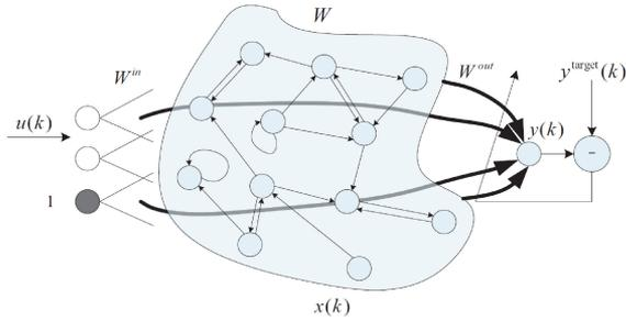
Fig. 20. RUL prediction of power MOSFETs based on ESN [111]. For the network training, the input weights  $W^{\text{in}}$  and the recurrent weights  $W$  are randomly generated. The output weights  $W^{\text{out}}$  are estimated by least-square methods.
