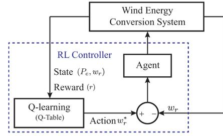
Fig. 13. Framework of RL in the MPPT controller of wind energy conversion systems [5], [138]. A Q-table is formulated to save the optimal generator rotor speed  $w_r^*$  to be performed given the current system state  $s_t$ , including the current electrical output power  $P_e$  and the generator rotor speed  $w_r$ .
