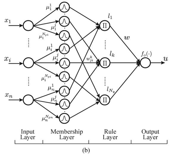
Fig. 10. FNN-based controller for a boost converter [100].  $x_1$  is the sliding surface  $S(x)$  and  $x_2$  is its differentiation,  $n = 2$ .  $\mu_i^j$  is the  $j$ th membership function for input  $x_i$ .  $w$  is the weight between layers. (a) Block diagram of the FNN-based controller for a boost converter. (b) FNN with a four-layer structure.
