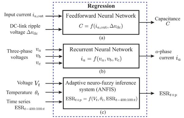
Fig. 15. Examples of model-free methods of system parameter identification with AI. (a) Capacitance identification of dc-link capacitor [88]. (b)  $a$ -phase current estimation for calculating the impedance measurement of power electronic system [108]. (c) ESR estimation in future  $p$  steps for supercapacitors [103].
