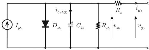
Fig. 16. Dynamic model of a PV panel for parameter identification with the model-based method [69]. System parameters include the input current  $I_{ph}$ , output current  $I_o$  ( $i_o(t)$ ), voltage  $v_{sh}$  across capacitor  $C_{sh}$ , resistor  $R_{sh}$ , p-n junction capacitance  $C_{sh}$ , and resistor  $R_s$ .
