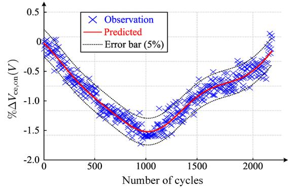
Fig. 21. Gaussian processes regression for the RUL prediction of IGBTs [119].
