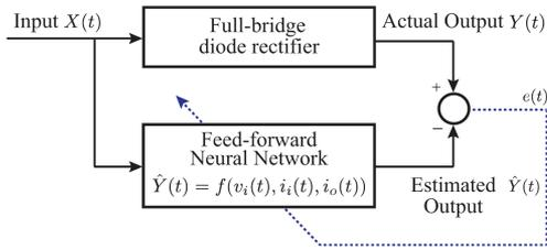
Fig. 18. FFNN for anomaly detection of a full-bridge diode rectifier. The inputs of the NN include input voltage  $v_i(t)$ , input current  $i_i(t)$ , and output current  $i_o(t)$ ; the output of the NN is output voltage  $v_o(t)$  [93].
