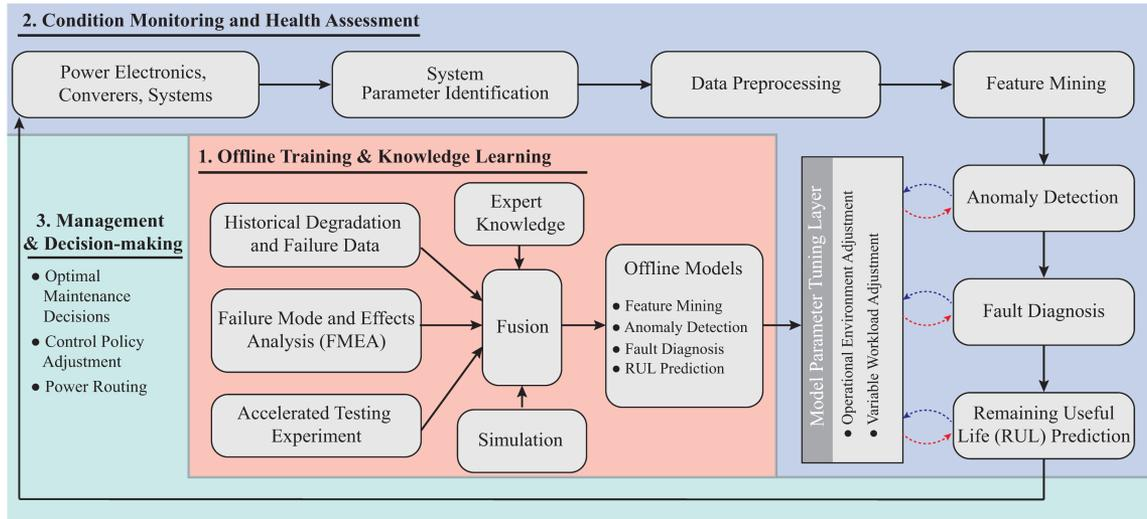
Fig. 14. Flowchart of maintenance in power electronic systems.
