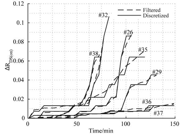
Fig. 17.  $k$ -means clustering method for discretization of filtered degradation paths of increment of drain-to-source ON-state resistance  $\Delta R_{DS(on)}$  of different power MOSFET devices #26, #29, #32, #35, #36, #37, #38 [131].
