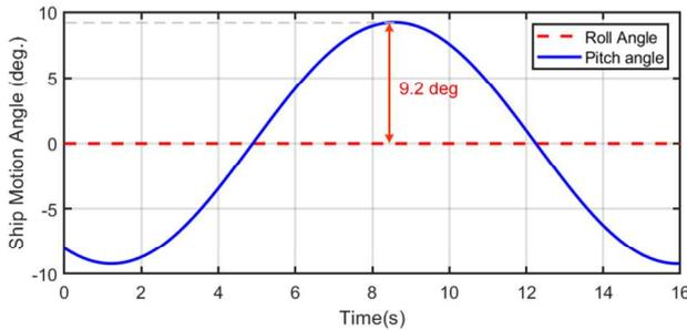
Fig. 6. The ship motion angles during the wave-encountering condition
