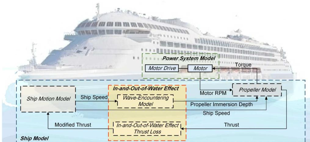
Fig. 1. The proposed interconnected model framework for investigating the in-and-out-of-water effect on the ship power system
