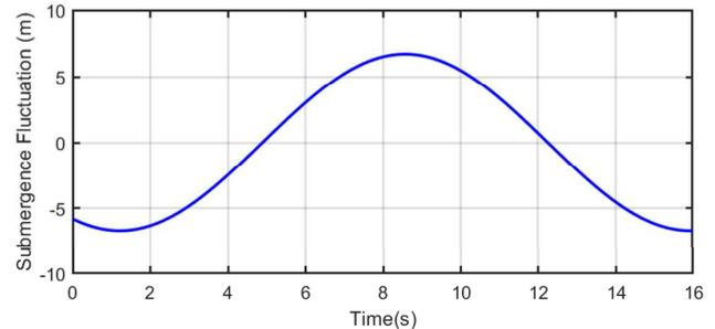
Fig. 7. The propellers submergence fluctuations during the wave-encountering condition
