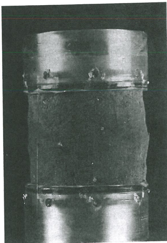
Fig. 1.17 Samples after rupture. A moraine clay sample and a sand sample after a deformation at about 15 %.
