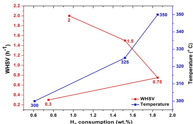
Fig. 7. H<sub>2</sub> Consumption during co-HDO experiments at different temperatures and WHSV.
