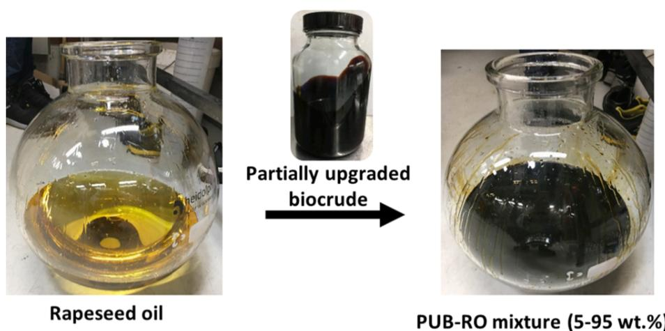
**Fig. 5.** Preparation of PUB-RO (5–95 wt%) blend as starting feed for the continuous co-HDO campaign on a fixed bed reactor.
