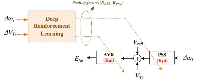
Fig. 2. Proposed coordinated control for AVR and PSS
