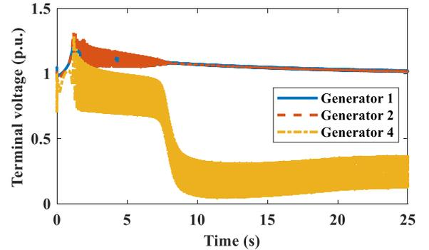
Fig. 4. Time-domain responses of rotor angle, rotor speed, accelerator power, and terminal voltage of the generators without DRL coordinator.
