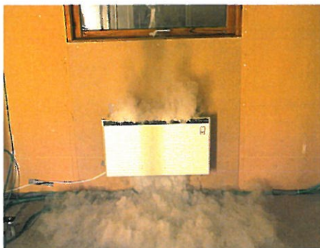
Figure 2. Development of stratified semi-radial jet from the ULV device.
