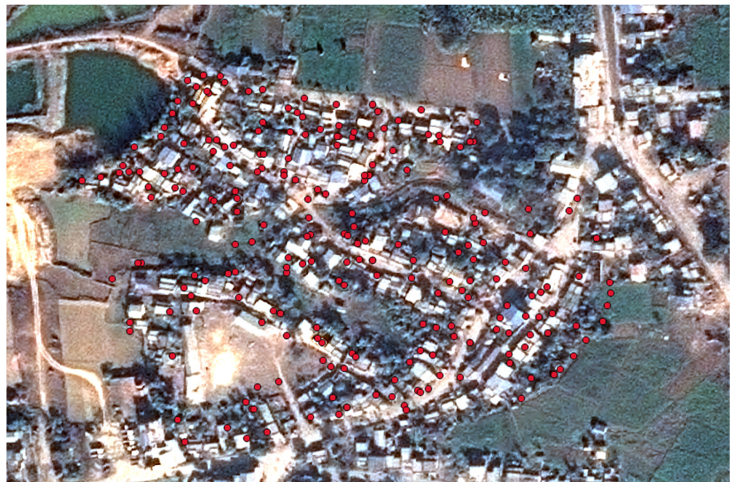
Figure 3. Identification of house/property in one of the compact settlements of Ratnanagar Municipality. The individual house location is shown with red-colored dots with satellite imagery in the background.
